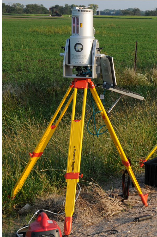
Figure 14: The Riegl LMS-Z620 survey LiDAR scanner is pictured here at Victory Road. It is mounted on top of a tripod at each scan location. Controlling the scanner is accomplished through RiScan Pro software which is installed on the laptop mounted on the tripod.
