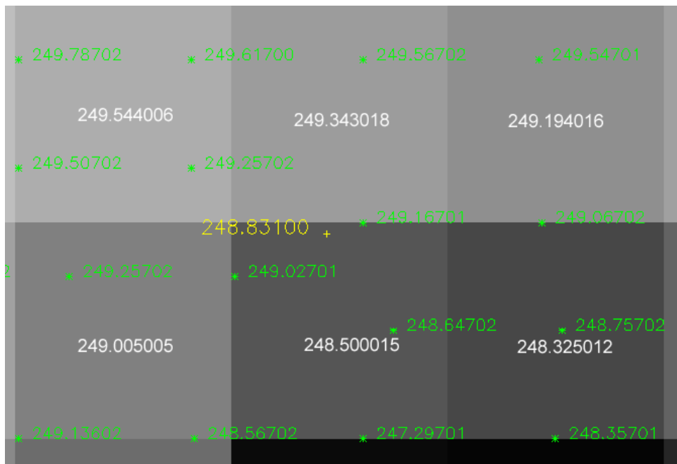
Figure 2-10. GPSBM “B276 Reset”, located in Lawrence, KS, is shown in the photo above. As an example of the inherent difficulty in using a point elevation (represented in yellow in the bottom graphic by “B276 Reset”), 2 meter DEM cells are show above in gray with corresponding values in white. The green asterisks represent the location and values of the LiDAR returns from which the DEM values are derived. A LiDAR vendor would likely not use this GPSBM as a checkpoint because of the uneven ground surrounding the checkpoint.
