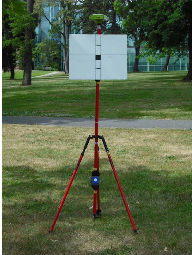
Figure 1. One of four Leica Geosystems HDS Twin-Target Poles used in this study. Shown with a) Javad Maxor Global Positioning System (GPS) unit attached at top for recording reference data (GPS center at 2.15 m height), and b) White board with black crosshair target used for rangefinder experiment (target center at 1.75 height).
