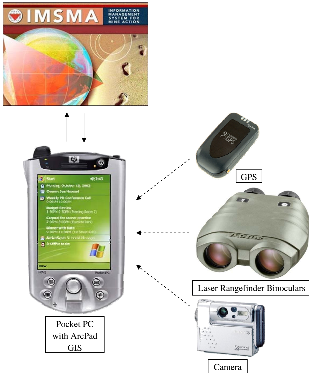
Figure 1. Mobile GIS system for humanitarian demining. Data are transferred via USB between PocketPC and IMSMA desktop software. The PocketPC receives data wirelessly via Bluetooth from the GPS, Laser Rangefinder Binoculars, and Camera data collection devices.
