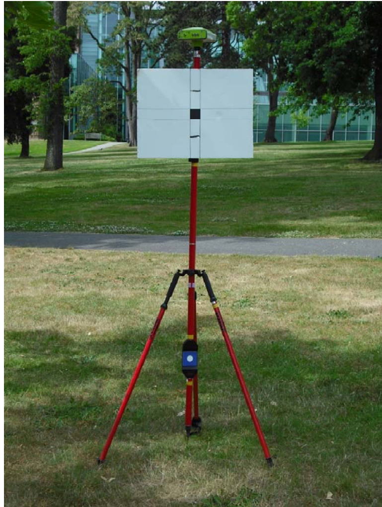
Figure 1. Leica Geosystems HDS Twin-Target Pole shown with a) Javad Maxor Global Positioning System (GPS) unit attached at top for recording reference data (GPS center at 2.15 m height).
