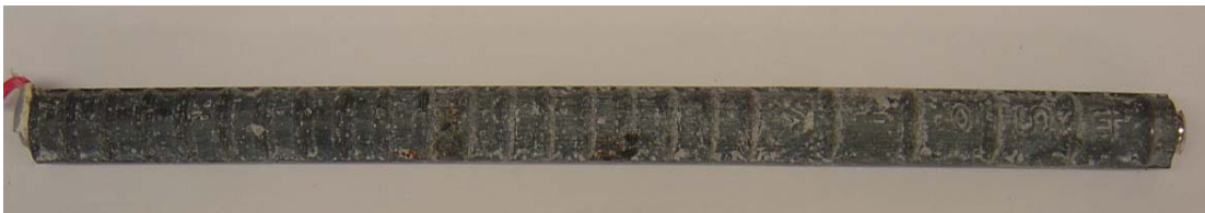
Figure 3.128 – Initiation Beam Test. Conventional steel in the top mat (B-N4-Hycrete-45N-3) showing slight corrosion.
