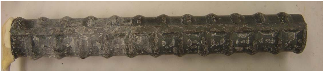
Figure 3.17 – Macrocell Test. Conventional steel from cathode specimen (M-Conv.-DCI45-3) showing no corrosion products at week 15.
