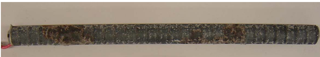
Figure 3.129 – Initiation Beam Test. Conventional steel in the top mat (B-N4-Rheocrete-45N-4) showing severe corrosion.
