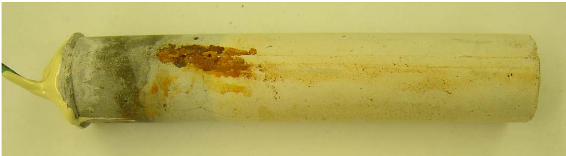
Figure 3.13 – Macrocell Test. Anode specimen (M-Conv.-NO45-1) with conventional steel showing stains on cracked mortar surface at week 15.
