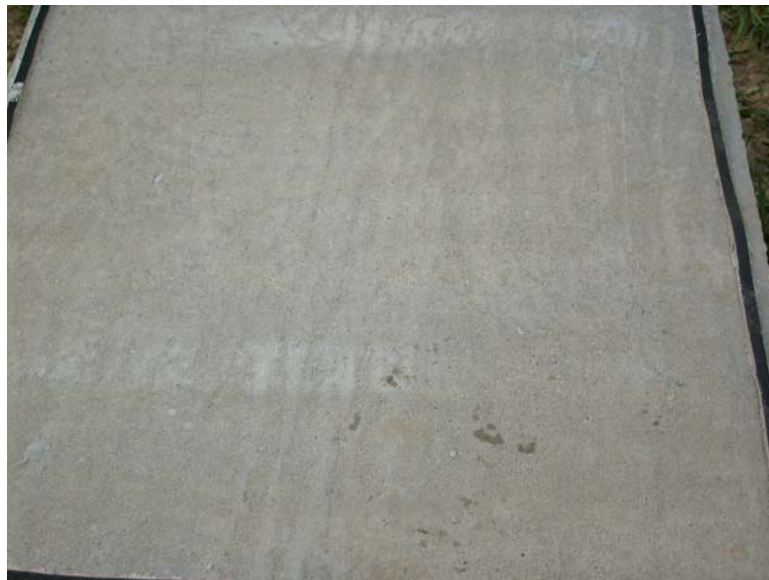
Figure 3.93 – Field test specimen ECR (1) at week 205, showing no cracking or staining of the surface.
