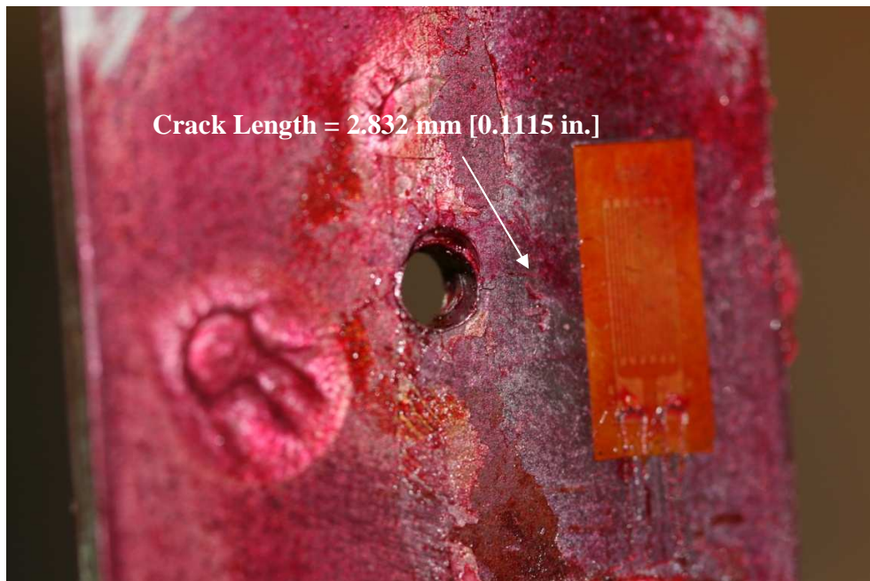
Figure D-12: Cracked specimen PICK 3 side 2, failed at 818,635 cycles
