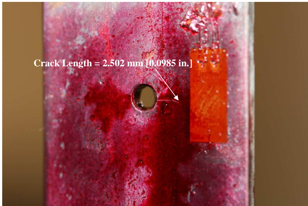
Figure D-14: Cracked specimen PICK 4 side 2, failed at 743,725 cycles
