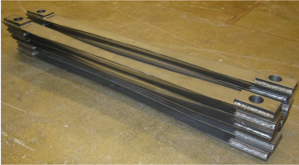
Figure 3-4 : 3.18mm [0.125in.] fatigue specimens, fabricated by Rice Precision Manufacturing, located in Baldwin, KS
