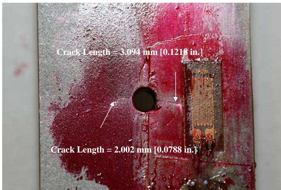
Figure D-7: Cracked specimen Control_12 side 1, failed at 195,220 cycles
