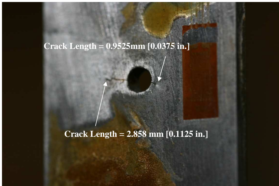
Figure D-16: Cracked specimen PICK 6 side 2, failed at 426,302 cycles
