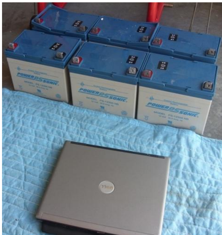
Figure 4.10: Six PowerSonic 12-volt, 35 ah deep cycle AGM batteries (laptop left in photo to show scale)
