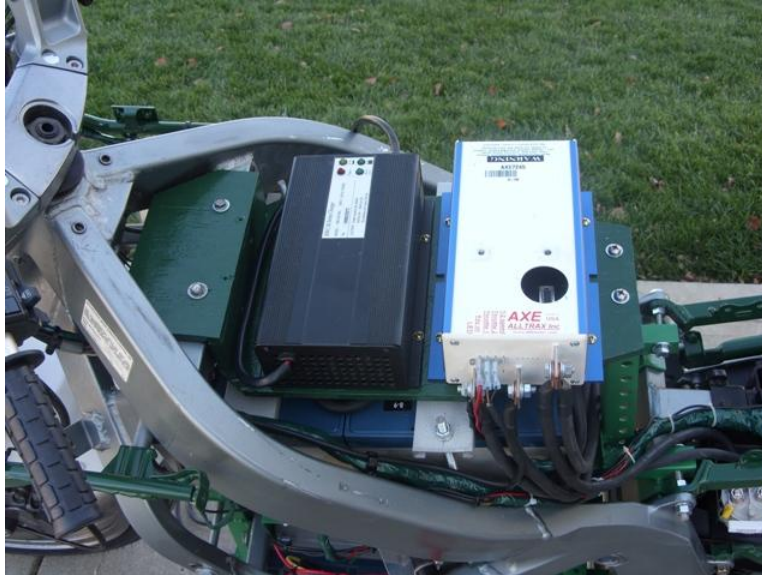
Figure 4.18: Mounting board showing motor controller and charger
