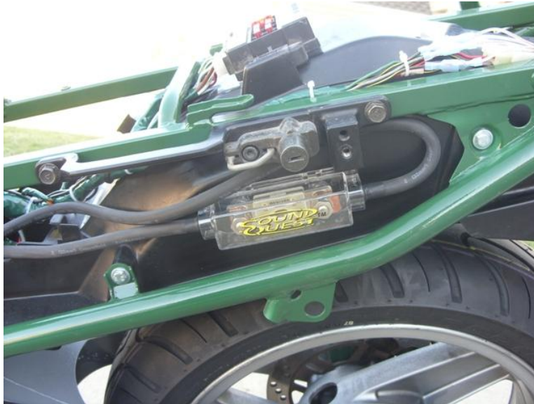
Figure 4.20: 400 amp main system fuse location and sample of the 2-AWG cabling
