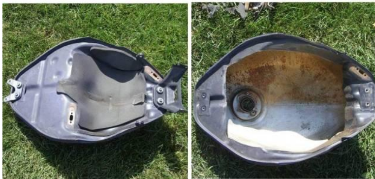
Figure 4.19: Before and after: fuel tank with bottom removed to make room for components
