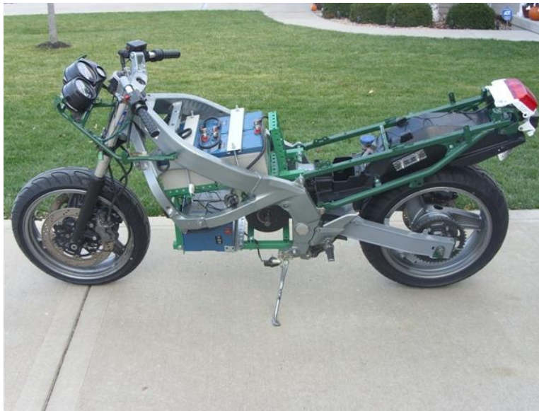
Figure 4.17: Fabricated sub frame with motor and batteries installed
