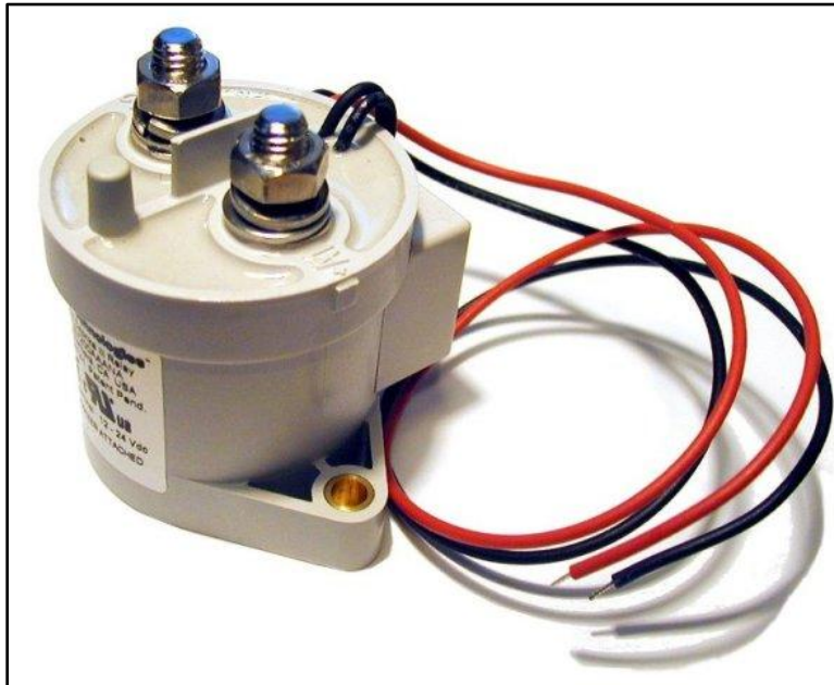
Figure 4.13: Kilovac EV200 Contactor by Tycho Electronics ( www.evsource.com , 2009)
