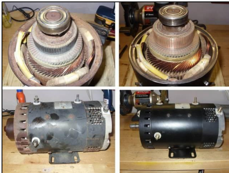
Figure 4.6: Looking left to right; before and after condition of 6.7" dia. electric motor
