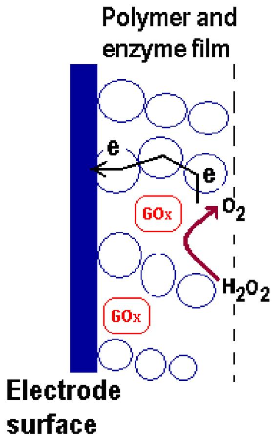
Figure 7: Schematic diagram of electrode modified with conducting polymer film
