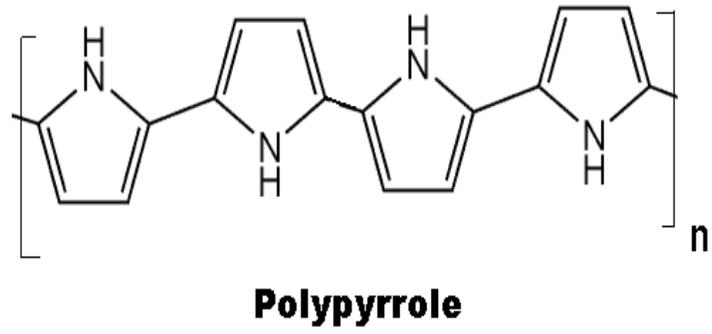
Figure 6: Structures of pyrrole and polymerized pyrrole (PPy)
