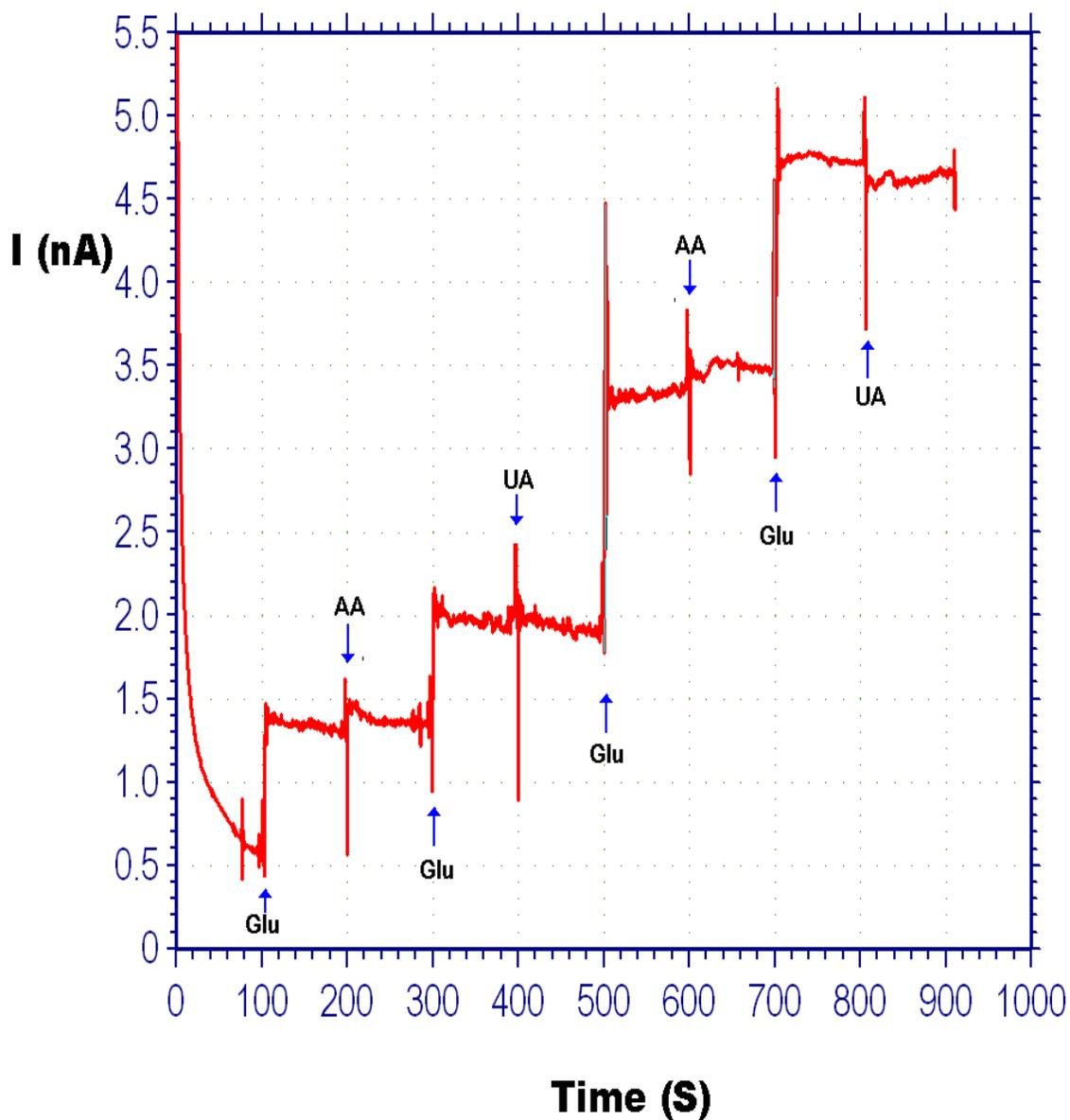
Figure 20: Typical current-time curve for 0.75% Nafion<sup>®</sup> coated Pt/PPy/Gox 25µm microelectrode upon sequential addition of 5.0mM D-glucose (Glu), 0.1 mM ascorbic acid (AA) and 0.1 mM uric acid (UA). Working electrode potential: +0.6V (vs. Ag/AgCl)
