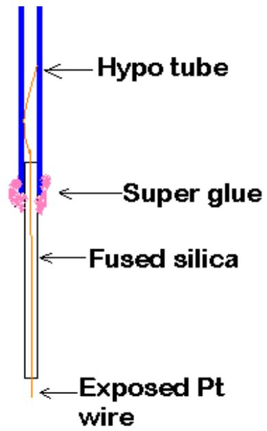
Figure 11: A schematic representation of 25µm diameter Pt- fused silica microelectrode
