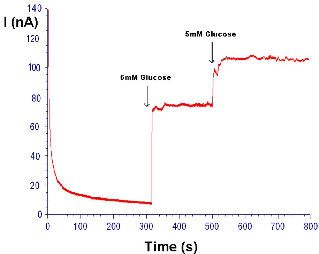
Figure 12: Typical current – time curve of 176 $\mu$ m non-conductive polymer based glucose sensor for two successive additions of 5.0mM glucose in PBS (pH 7.4, 50mM). Sensors were kept at +0.6V constant potential (vs. Ag/AgCl).
