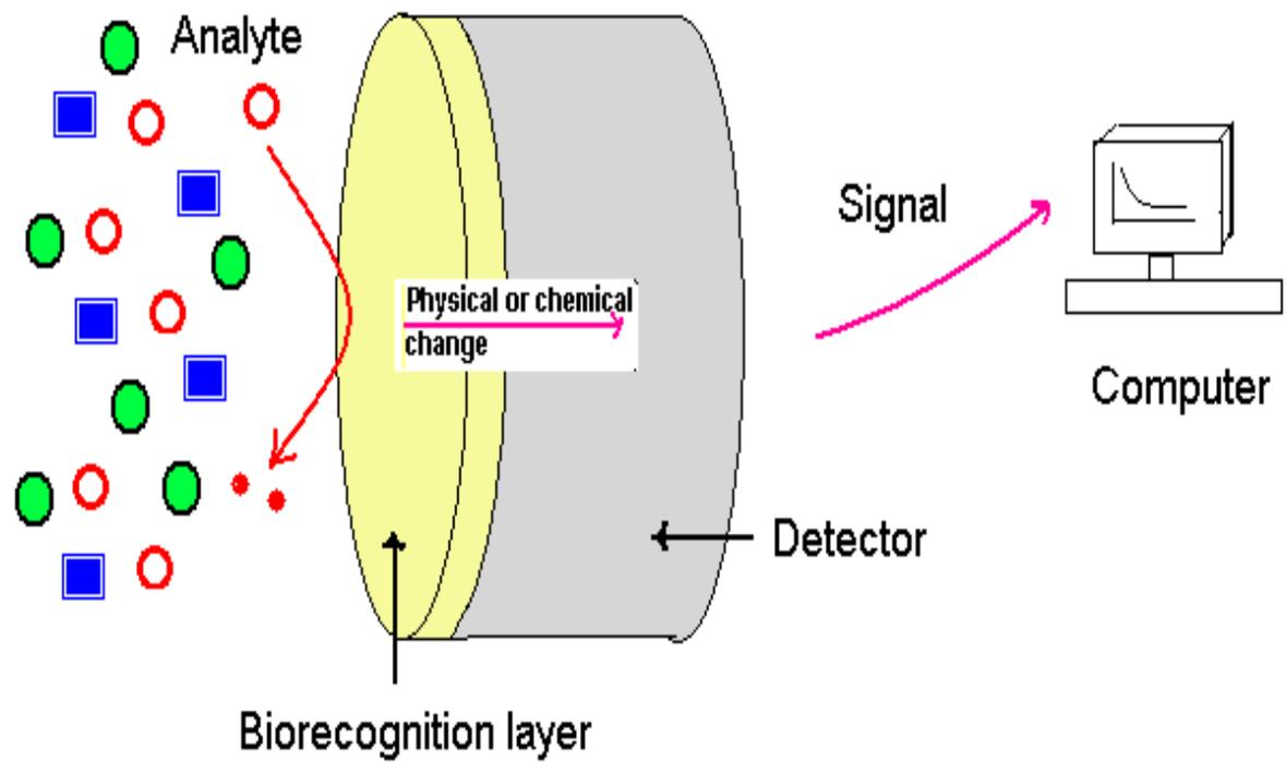
Figure 4: Schematic representation of a biosensor.
