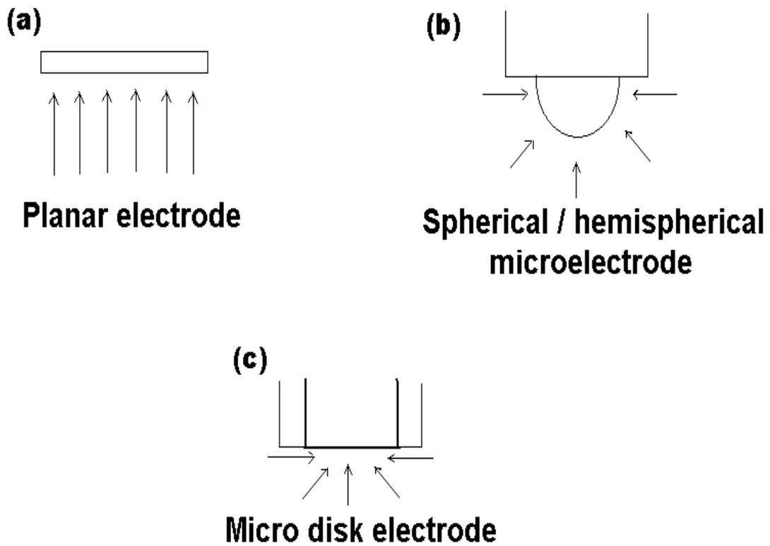
Figure 3: Illustration of analyte diffusion fields. (a) Linear diffusion field at a planar electrode, (b) Spherical diffusion field at a spherical or hemispherical microelectrode and (c) Spherical diffusion field at a disk microelectrode.
