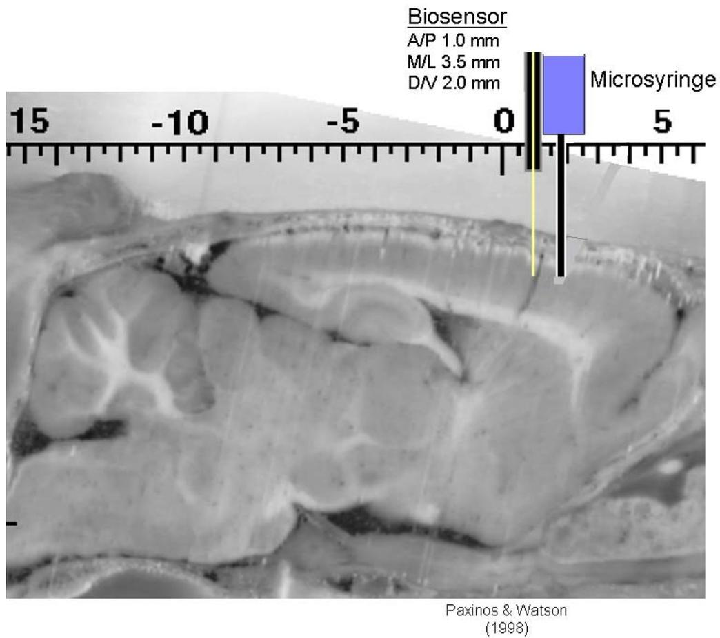
Figure 23: Diagram of 25µm Pt/PPy/GOx sensor and microsyringe implantation on a rat cortex.
