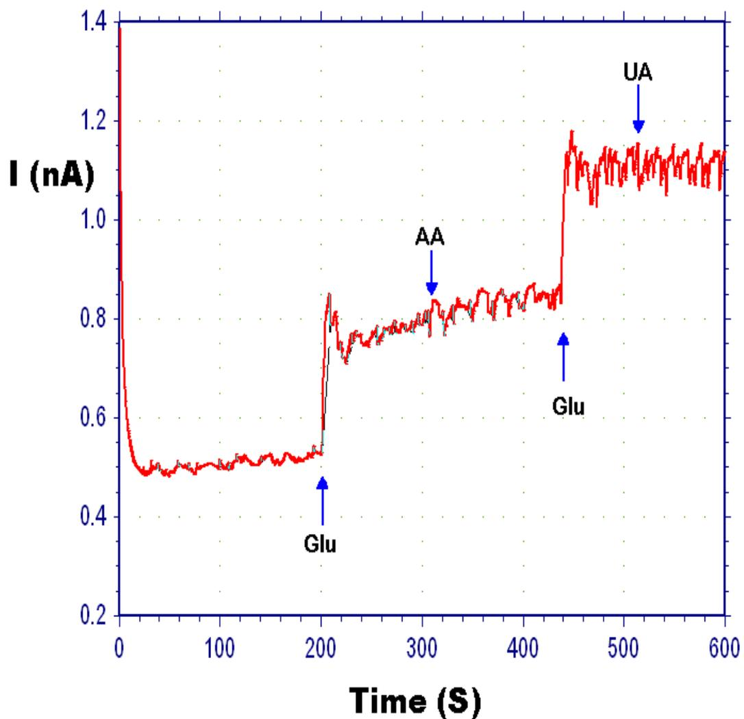
Figure 15: Current-time curve of 176µm glucose sensor for successive injection of 5.0mM glucose 0.1mM ascorbic acid and 0.1mM uric acid in pH 7.4 PBS solution. Sensors were kept at +0.6V (vs. Ag/AgCl)
