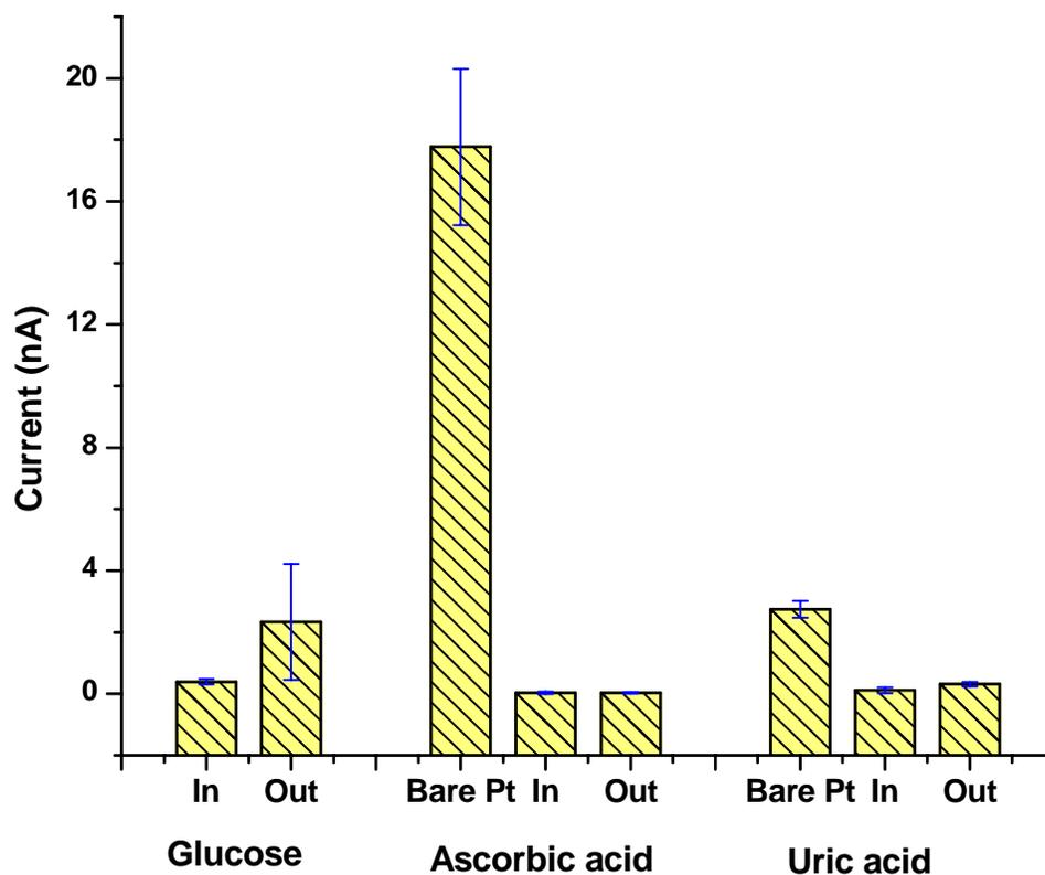
Figure 18: Response of 5% Nafion directly coated (In) 25µm electrodes and Nafion coated after the enzyme/pyrrole layer (Out) and 25µm bare Pt electrodes against 0.1mM glucose, 0.1mM ascorbic acid, and 0.1mM uric acid additions. Working potential is +0.6V against Ag/AgCl reference. (N=4-6 sensors)
