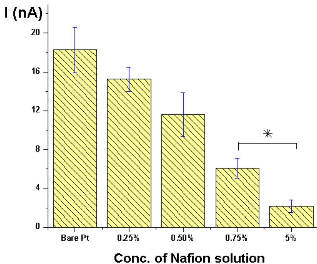
Figure 19: Current generated by oxidation of 0.1mM  $H_2O_2$  against 25 $\mu$ m microelectrodes coated different concentrations (weight %) of Nafion<sup>®</sup>. (\*  $P > 0.05$ ) (n=4-6)
