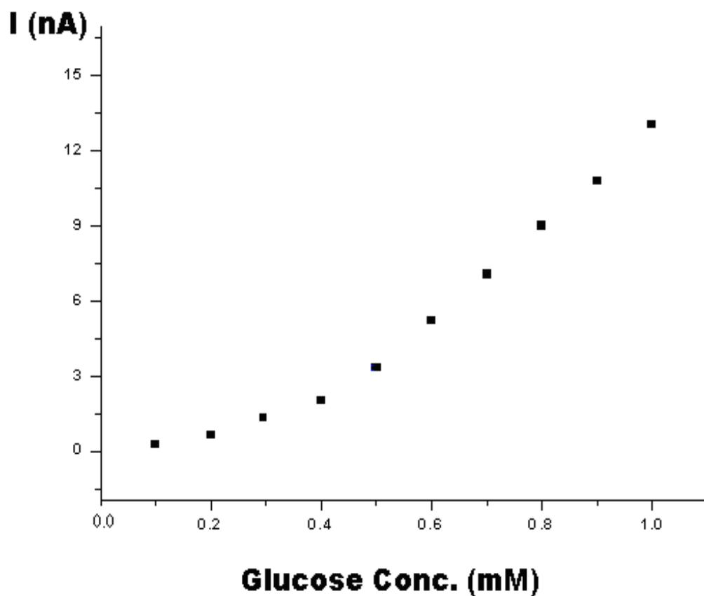
Figure 14: Response of 176µm glucose sensor against standard addition of glucose to pH 7.4 PBS solution. The final concentration of glucose in the cell after addition of glucose is from 0.1mM glucose to 1.0mM. Sensors were kept at +0.6 V (vs. Ag/AgCl) (n=2) ( $R^2$  for 0.4-1.0mM is 0.9969)
