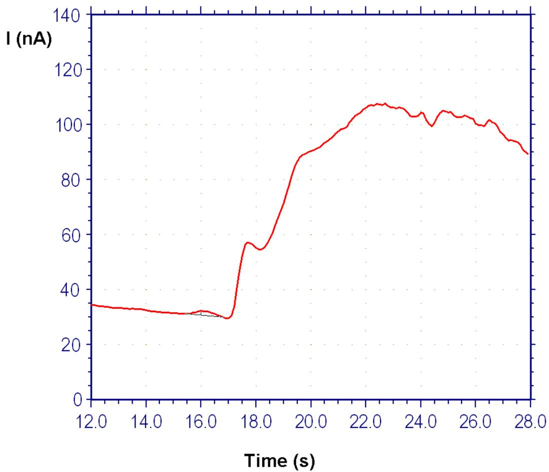
Figure 13: Typical current – time curve of 176 $\mu$ m non-conductive polymer based glucose sensor for flow cell analysis. Current increase is due to the additions of 250mM glucose. Sensors were kept at +0.6V constant potential (vs. Ag/AgCl).
