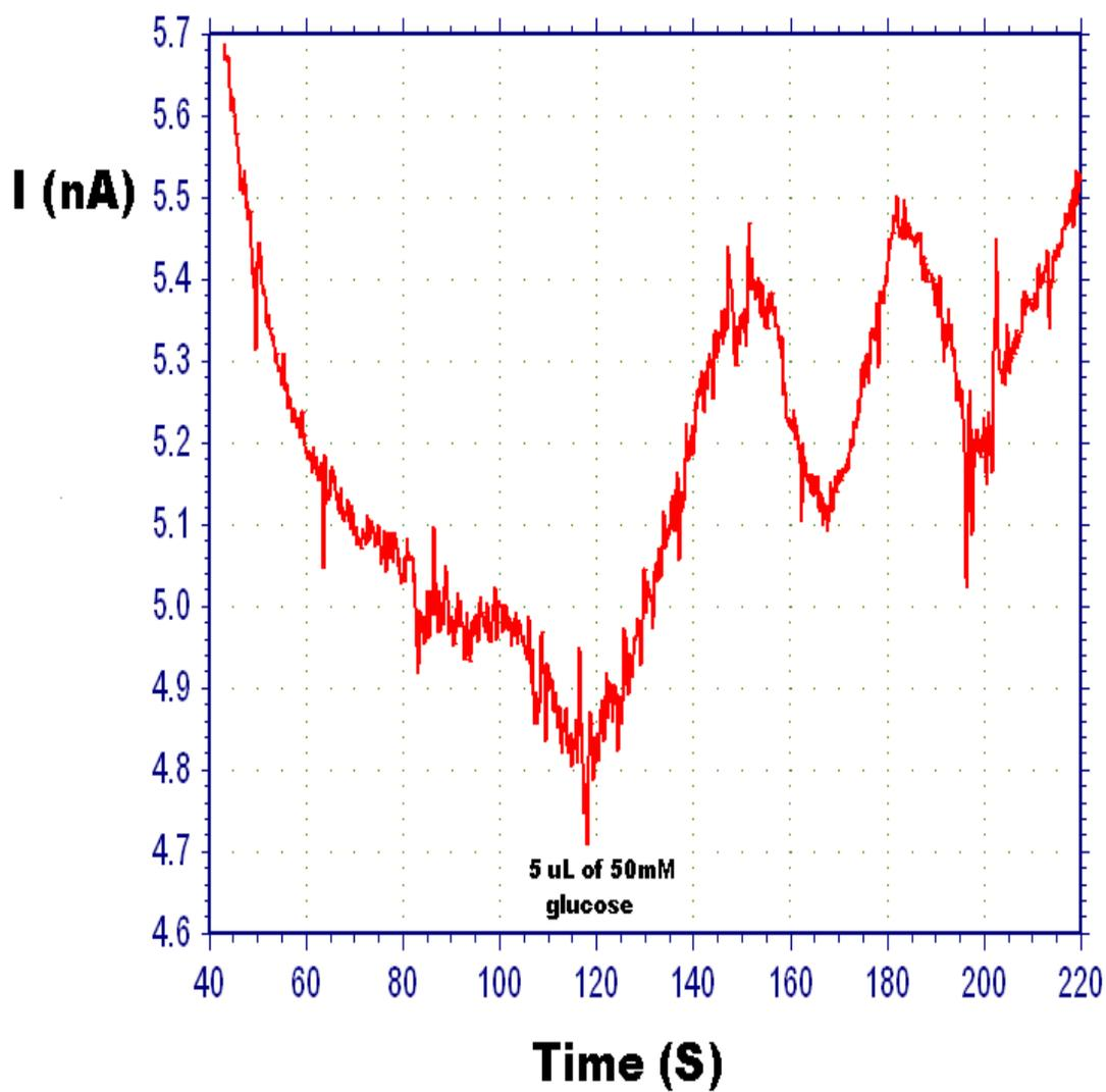
Figure 24: *In-vivo* Current Response of 25 μm Pt/PPy/GOx sensor after injecting 0.25 mM glucose. (5 μL of 50 mM solution of glucose) Initially, the sensor had a decreasing background current and after the glucose was injected the current signal was increased. Then, the current signal was fluctuated between 5.5 -5.1 nA.
