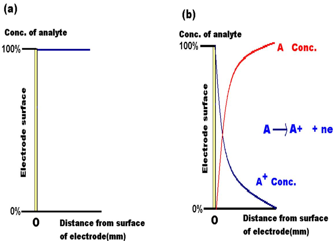
Figure 2: Concentration profiles of an analyte in the vicinity of a planar electrode (a) Concentration profile of an analyte (A) before a potential step is applied. (b) Concentration profiles of analyte (A) and oxidized form (A<sup>+</sup>) of analyte during a potential step to peak potential (E<sub>p</sub>).
