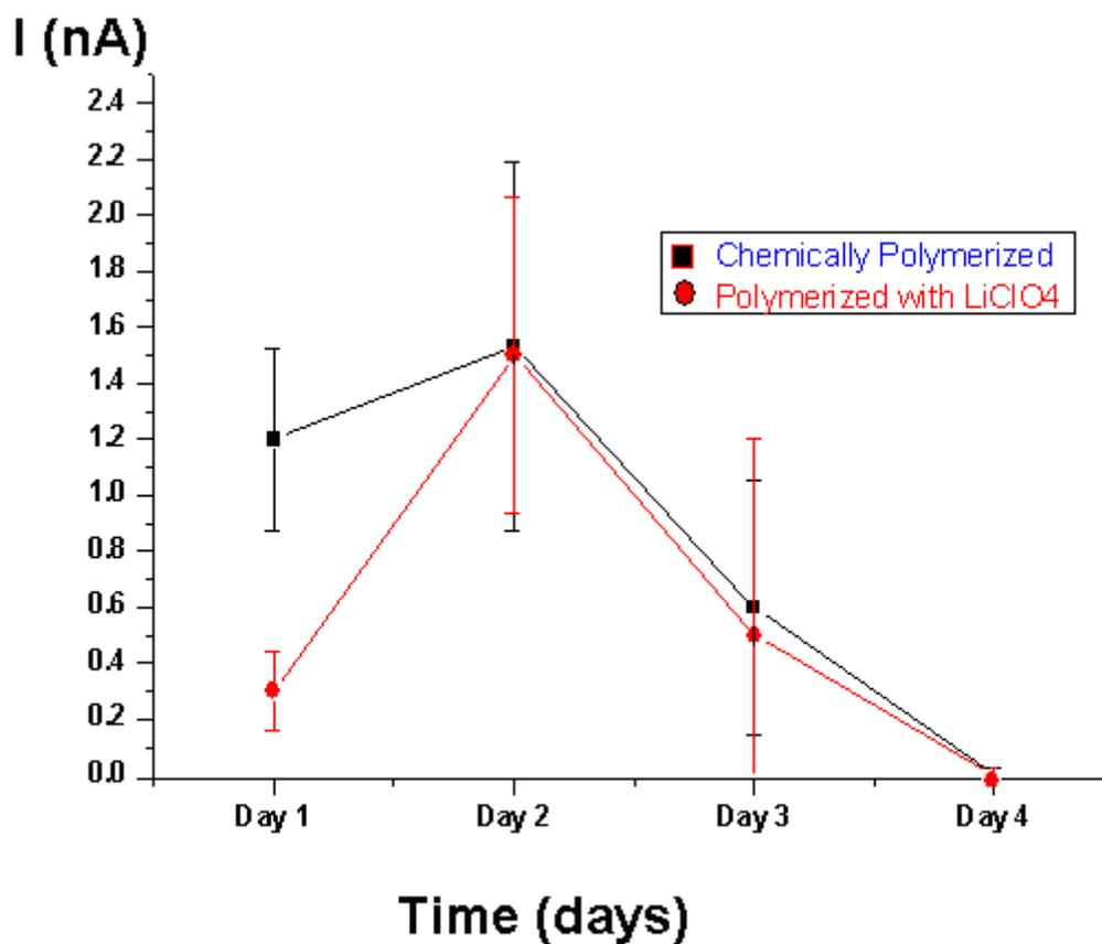
Figure 17: Stability comparison of 25 $\mu$ m Pt/PPy/GOx sensors polymerized electrochemically with LiClO<sub>4</sub> and 25 $\mu$ m Pt/PPy/GOx sensors polymerized chemically/ naturally without LiClO<sub>4</sub> by addition of 5mM glucose in PBS (pH 7.0, 0.1M). Sensors were kept in +0.6 V (vs. Ag/AgCl) (n=3)
