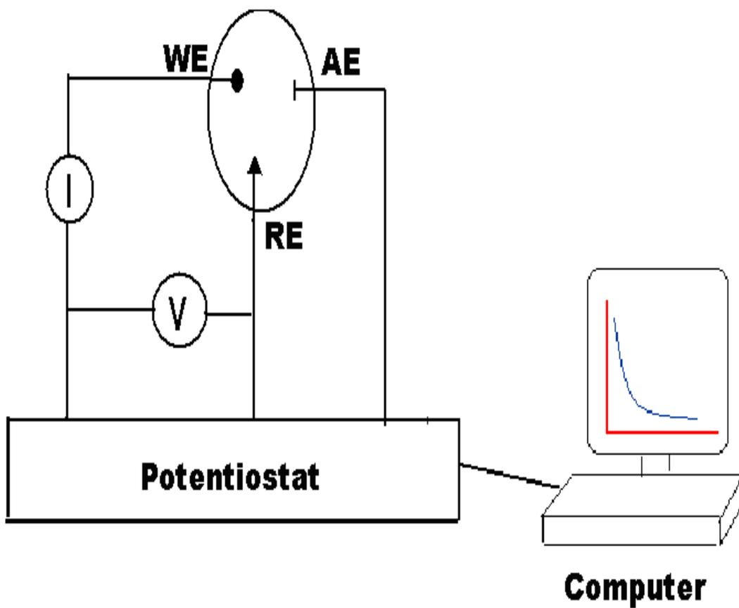
Figure 9: Basic components of the *in-vitro* amperometric experimental set up used in this research.
