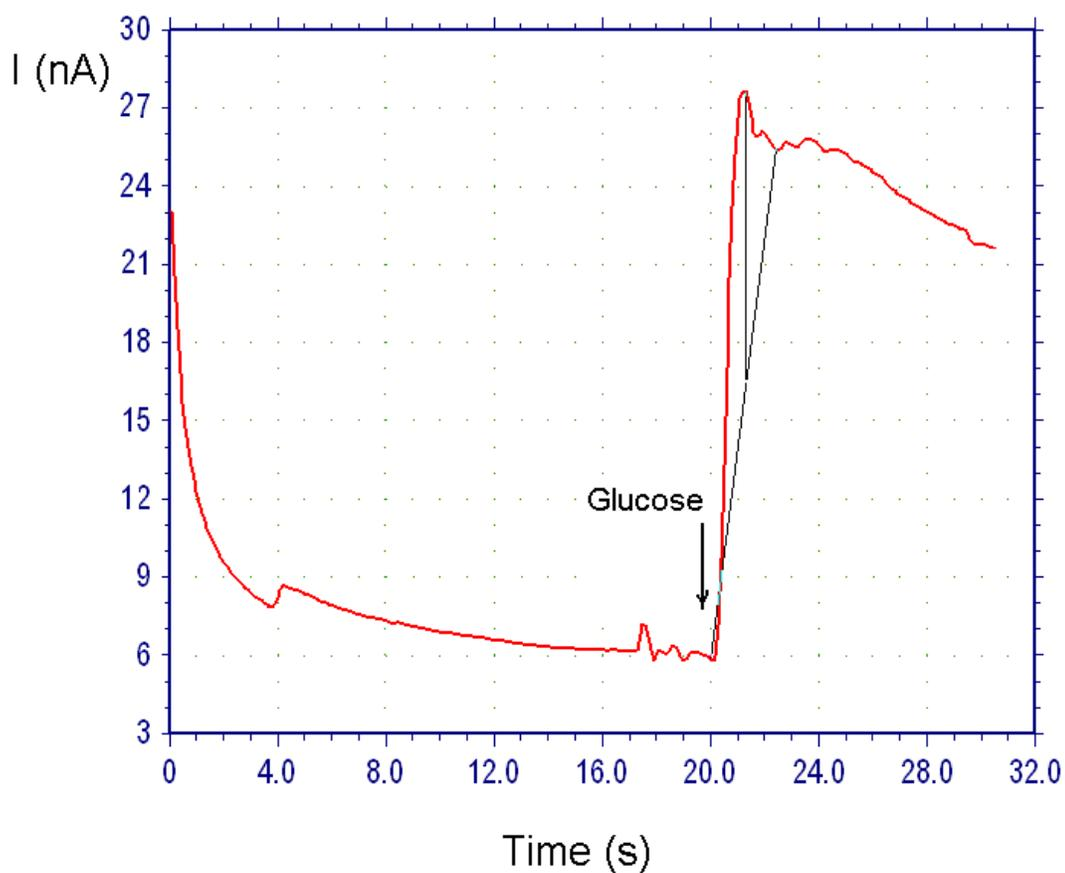
Figure 21: Typical current – time curve of 25 $\mu$ m Pt/PPy/GOx glucose sensor for flow cell analysis. Current increase is due to the additions of 250mM glucose at 20.0s. Sensors were kept at +0.6V constant potential (vs. Ag/AgCl). (n =6) The average time for the glucose sensor to go from 10% to 90% of peak amperometric signal was  $1.4 \pm 0.5$  seconds.
