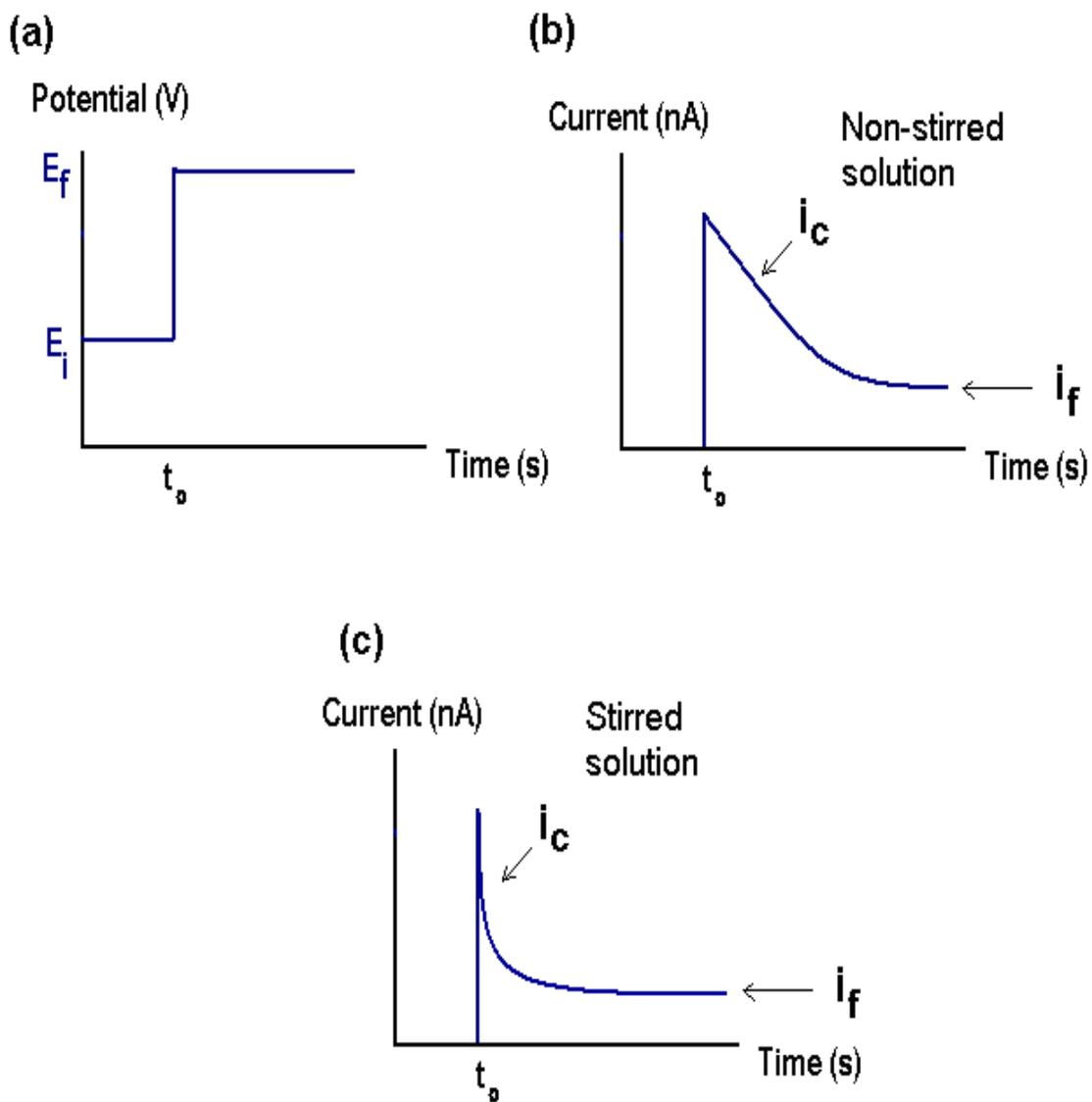
Figure 8: Illustration of the current change (b), (c) measured due to the oxidation or reduction of an analyte during a potential step (a) ( $i_c$  – charging current,  $i_f$  – faradaic current)
