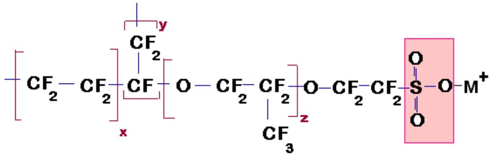
Figure 5: Chemical structure of Nafion<sup>®</sup> where, selected group is either carboxylic acid or sulfonic acid group and M<sup>+</sup> is a metal ion in the neutral form or H<sup>+</sup> ion in the acidic form.
