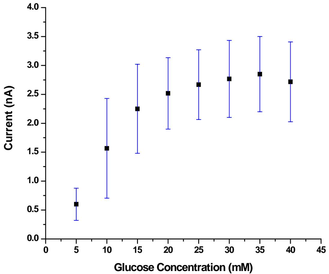
Figure 22: Calibration plot of 0.75% Nafion coated 25 $\mu$ m Pt/PPy/GOx biosensor against standard additions of glucose concentrations from 5mM up to 45mM in PBS (pH 7.0, 0.1M) (n=3) The sensors had linear response to glucose from 5mM to 15mM ( $R^2 = 0.9999$ ).
