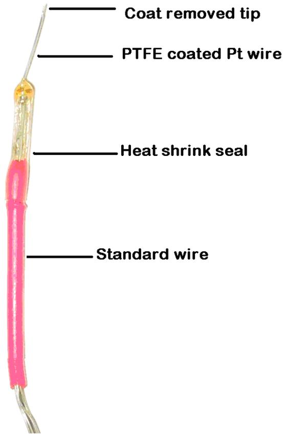
Figure 10: Pt wire type electrode (176 $\mu$ m diameter)
