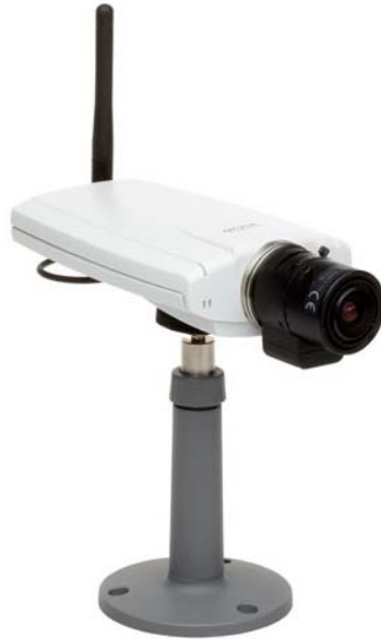
Figure 3.6: AXIS 211W IP Camera
