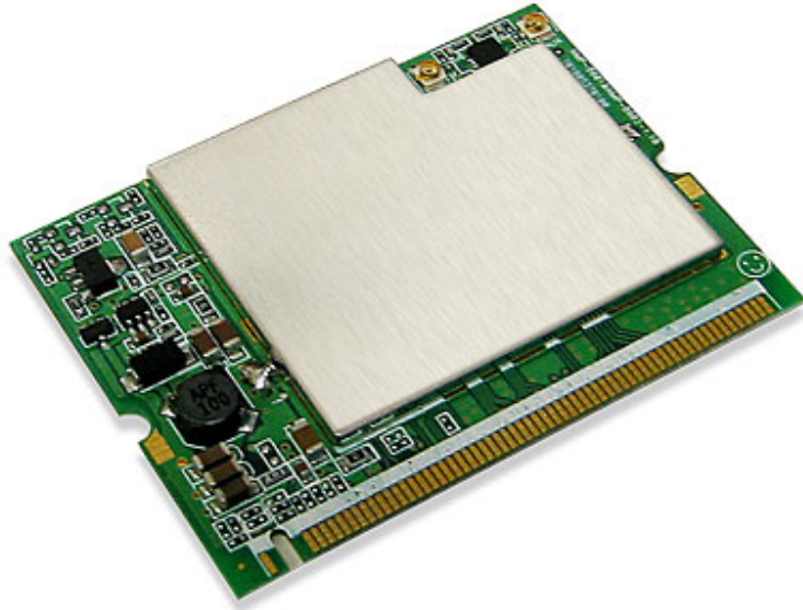
Figure 3.11: EMP 8602 Mini Wireless Card
