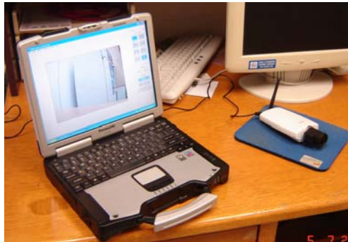
Figure 4.21: IP Camera in Ad-Hoc Mode with User Interface Node
