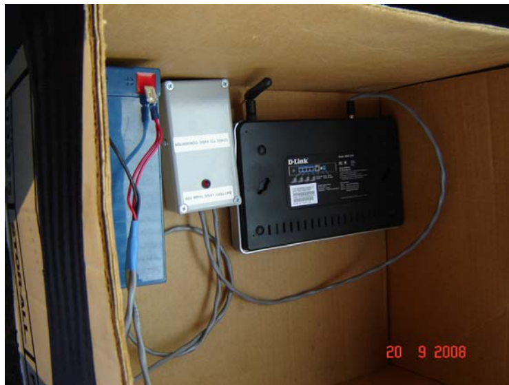
Figure 5.12: The Access Point and the Battery
