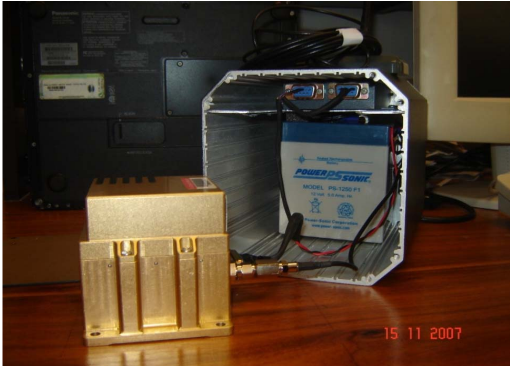
Figure 3.5: Assembly of the Wireless AHRS Unit
