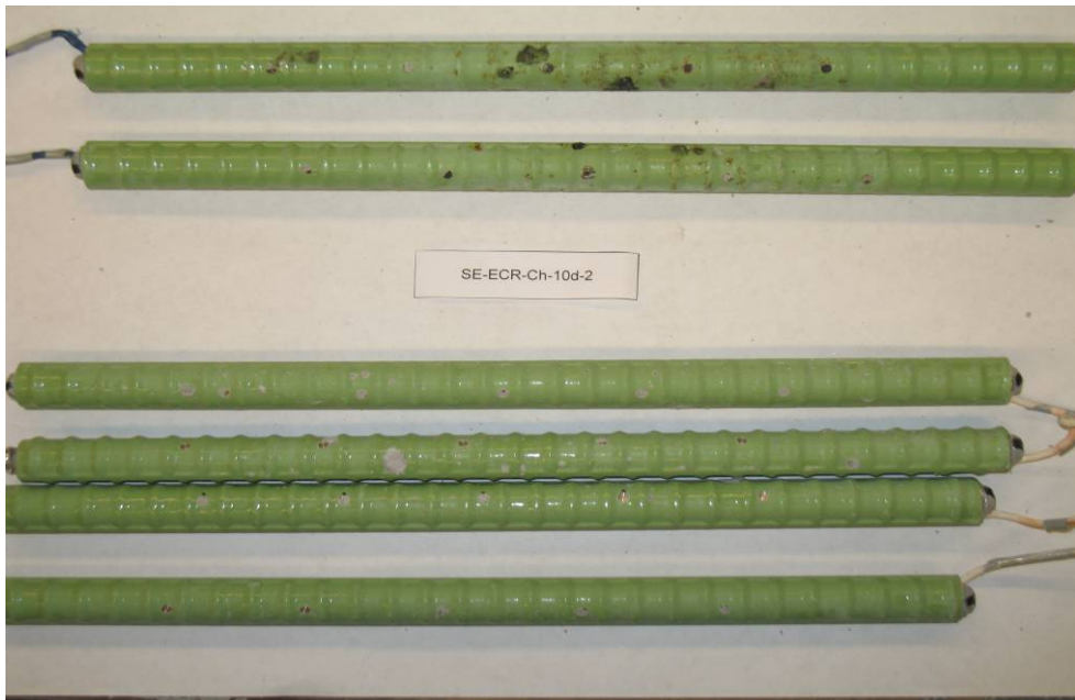
Figure 3.137 – Top and bottom bars of the ECR(Chromate)-10h-45-2 specimen at autopsy (before disbondment test). Top bars are shown at the top of the figure and bottom bars are show at the bottom of the figure.
