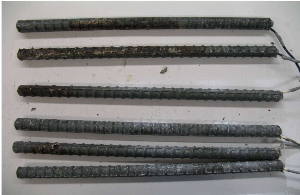
Figure 3.135 – Top and bottom bars of the Conv.-45-3 specimen at autopsy. Top bars are shown at the top of the figure and bottom bars are shown at the bottom of the figure.
