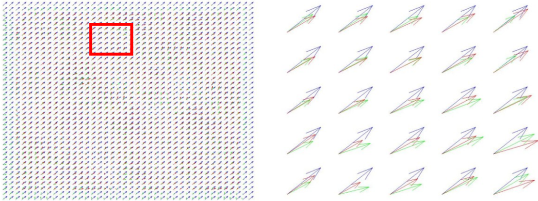
Figure 6.4: Joint Display (left) of Motion Analysis Results between the Pair of Translated Diagonally by 2 Pixels Images and its Magnified Version (right). The noise constant \alpha = 0.2 . A magnified view of the vectors from within the rectangular window is marked by the red rectangle on the left image. Color Code: \rightarrow True Motion diagonally by 2 pixel; \rightarrow Iterative OF algorithm estimated vectors; \rightarrow One-step algorithm estimated vectors.
