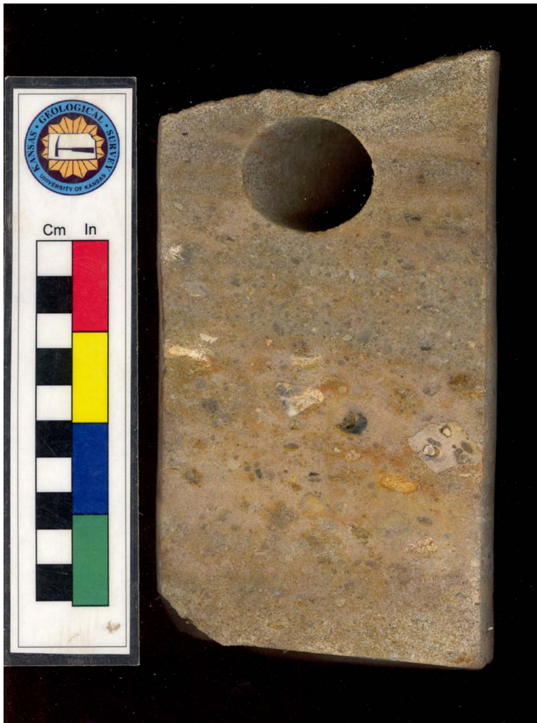
Figure 2.12. Conglomeratic Sandstone Facies – Core sample from 4135-4135.5 feet in the Thompson A2 (S3-T17S-R21W, Ness County, Kansas). Clast lithology is highly variable, similar to sample from Pfaff 3 core.
