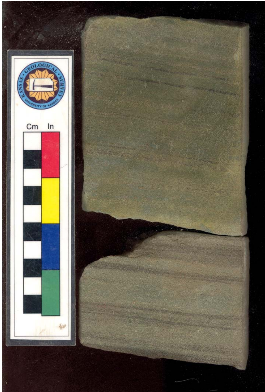
Figure 2.8. Cross-Laminated Sandstone Facies – Core sample from 4111.5-4112 feet in the Thompson A2 (S3-T17S-R21W, Ness County, Kansas).
