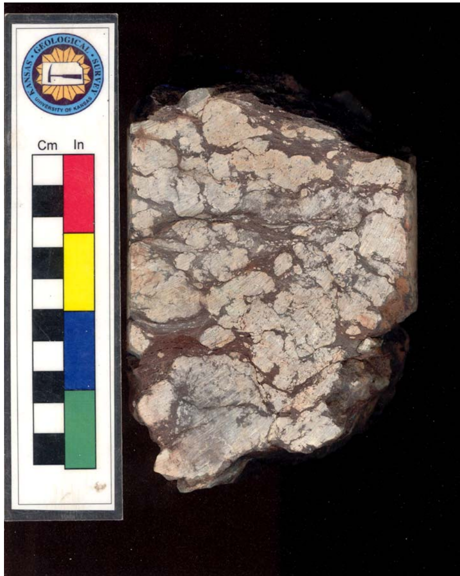
Figure 2.15. Variegated Silty Mudstone Facies – Core sample from 4139.5-4140 feet in the Thompson A2 (S3-T17S-R21W, Ness County, Kansas). Example of calcrete or caliche in a soil that formed in a carbonate rich rock. The sample formed in the top of a wackestone-packstone bed.
