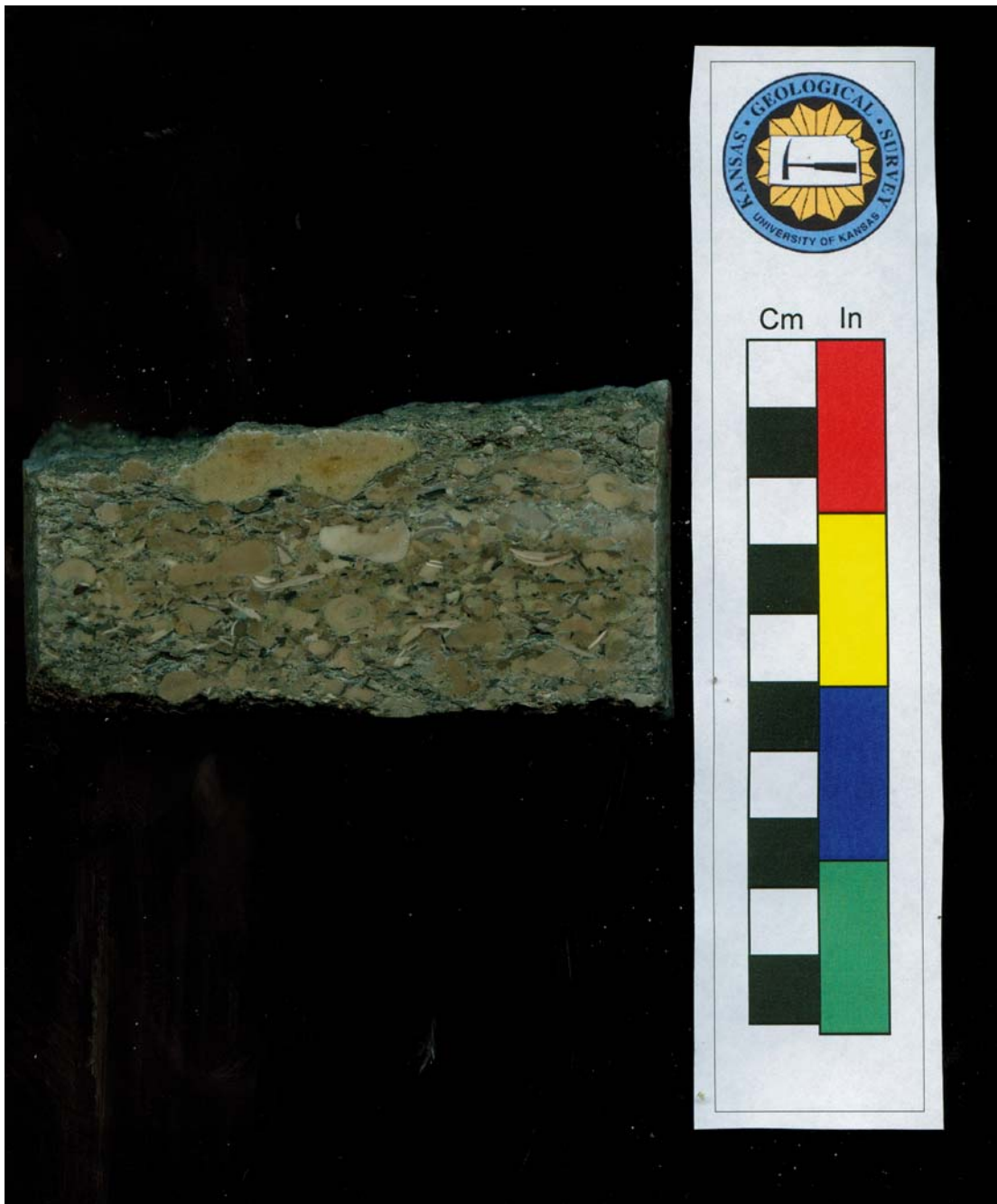
Figure 2.5. Skeletal Packstone to Grainstone Facies – Core sample from 4141.6-4141.75 feet in the Thompson A2 (S3-T17S-R21W, Ness County, Kansas). Note presence of aligned brachiopods and gastropod fragments. Large intraclasts located at top of sample.
