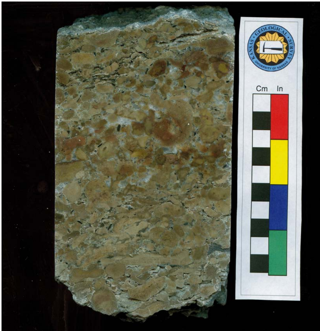
Figure 2.6. Skeletal Packstone to Grainstone Facies – Core sample from 4141.75-4142.3 feet in the Thompson A2 (S3-T17S-R21W, Ness County, Kansas). Abundant intraclasts with spar pore filling cement. Reddening of grains is interpreted as the result of post-depositional weathering.
