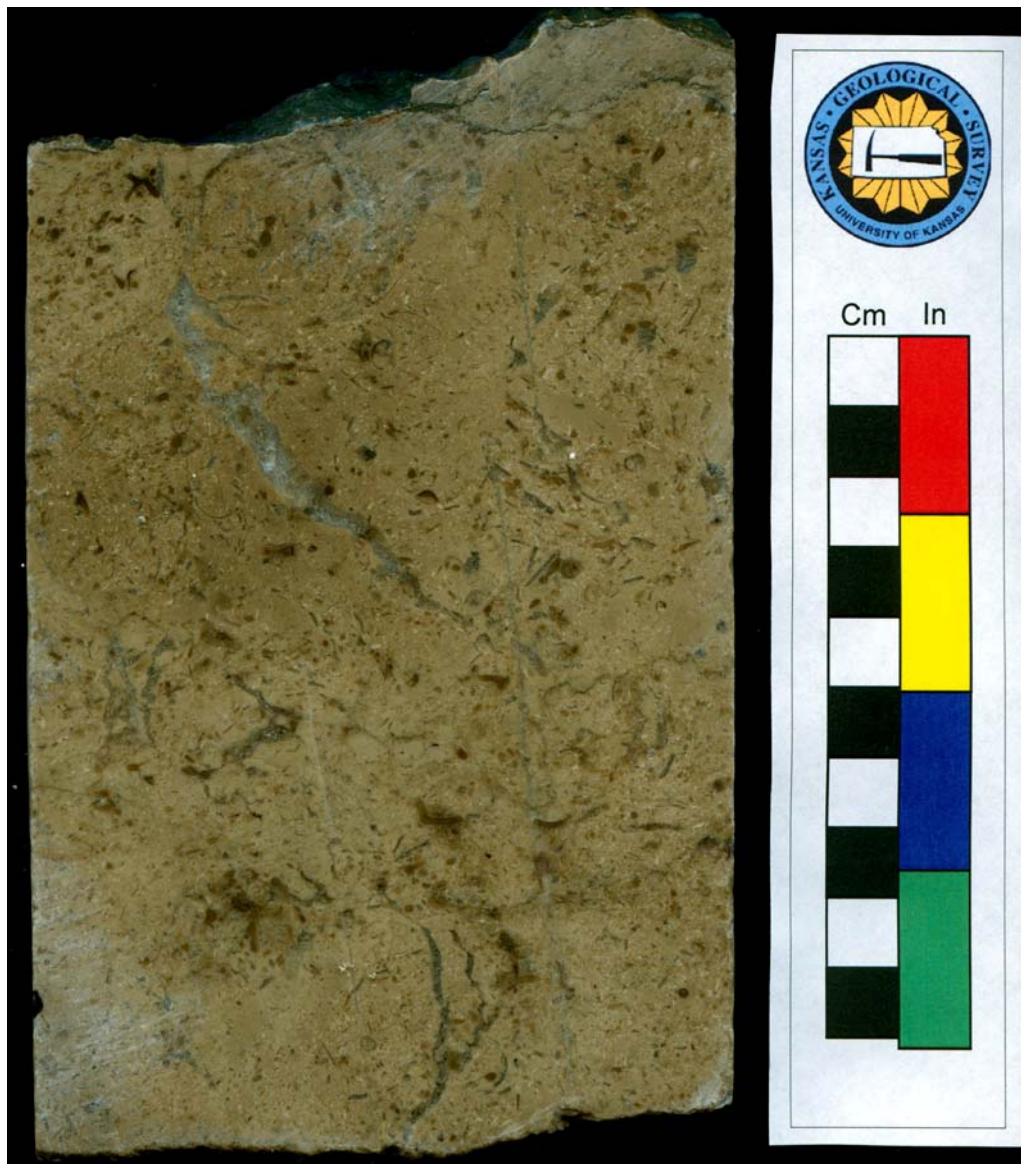
Figure 2.4. Carbonate Wackestone to Packstone Facies – Core sample from 4253.7-4254.1 in the Wegele A1 (S21-T18S-R22W, Ness County, Kansas).
