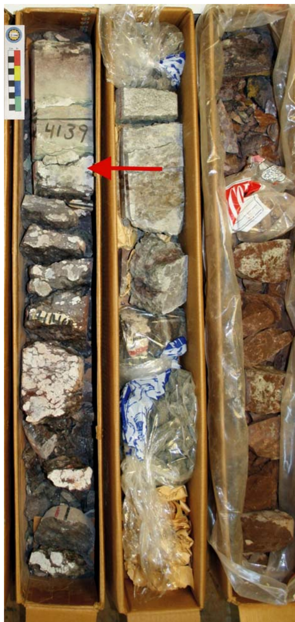
Figure 4.2. Core photograph of interpreted sequence boundary (SB2), indicated by the red arrow. Note caliche development in variegated silty mudstone facies (interpreted as a paleosol) sharply overlain by conglomeratic sandstone facies. Example is from 4128.6 feet to 4155.0 feet in Thompson A2 (S3-T17S-R21W, Ness County, Kansas).
