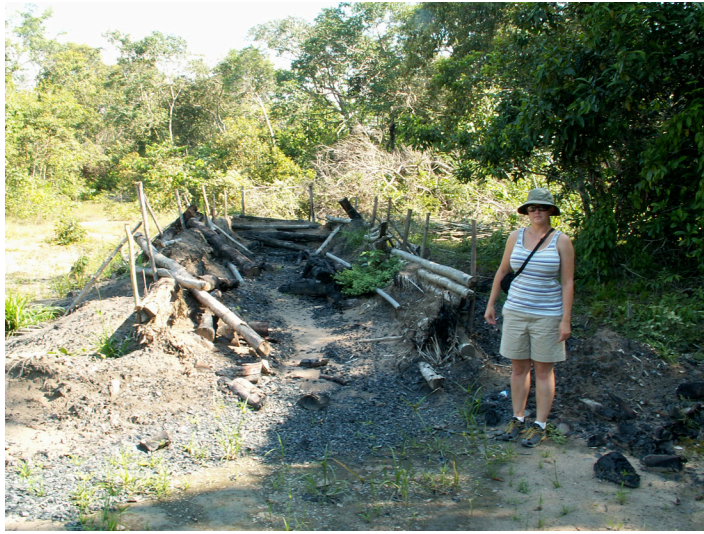
Figure 1.4 Modern primitive charcoal production sites. The first photograph is a log kiln where whole trees are buried and then burned with low levels of oxygen. The resulting charcoal is then mixed with soils in home garden plots and subsistence farms. We were able to find several of these trough-style kilns at the same farm. Apparently, the landowner builds a new one at the site of his most recently cleared field site. The area in the background of this photograph served as the source of the trees for this kiln. Undoubtedly this newly cleared site will become his next field. The second photograph is a clay charcoal kiln. Wood is placed inside and ignited and then the doorway is sealed to prevent the entry of oxygen. This charcoal is then sold to families who use it for cooking.
