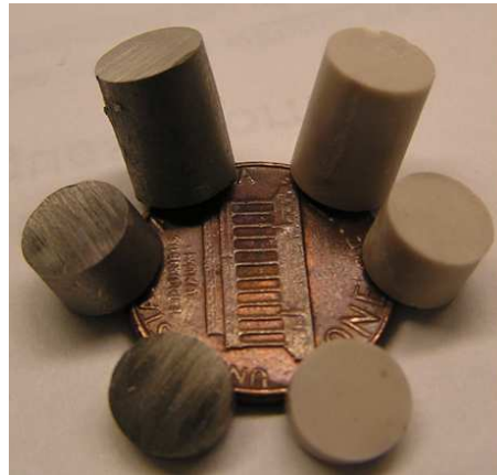
Figure 5-6. Photograph of the pure Ni (dark) and pure BaTiO 3 (white) specimens of different thicknesses (2mm, 5mm, 10mm)
