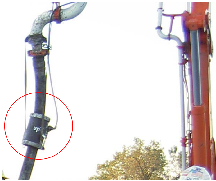
Fig. 5.5 – Bladder valve used to restrict and stop concrete flow through the concrete pump. The bladder valve works by compressing the discharge hose to restrict flow of the concrete.
