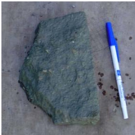
Fig. 5.13 – Example of a large coarse aggregate particle taken from the LC-HPC likely resulting in pumping difficulties.
