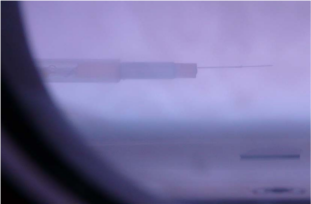
Figure 5.16: Photographs of a probe positioned to measure the presheath (Top, 100% N 2 , 15 mTorr, 50 W) and the bottom of the bulk of the plasma (Bottom, He plasma, 50 mTorr, 100 W).
