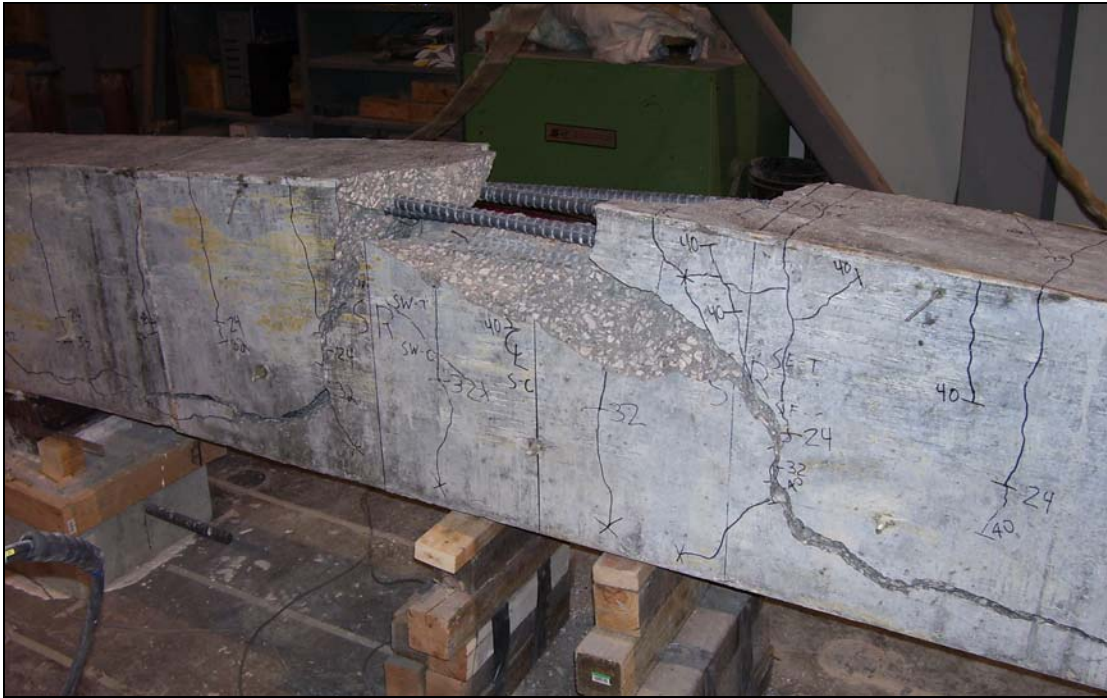
Figure B.18 – Specimen 8-8-OC0-2.5 at the conclusion of the test
