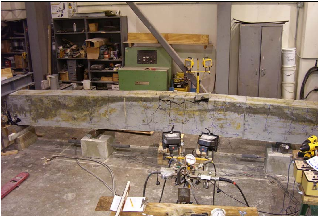
Figure B.19 – Specimen 8-8-OC1-2.5 at the conclusion of the test
