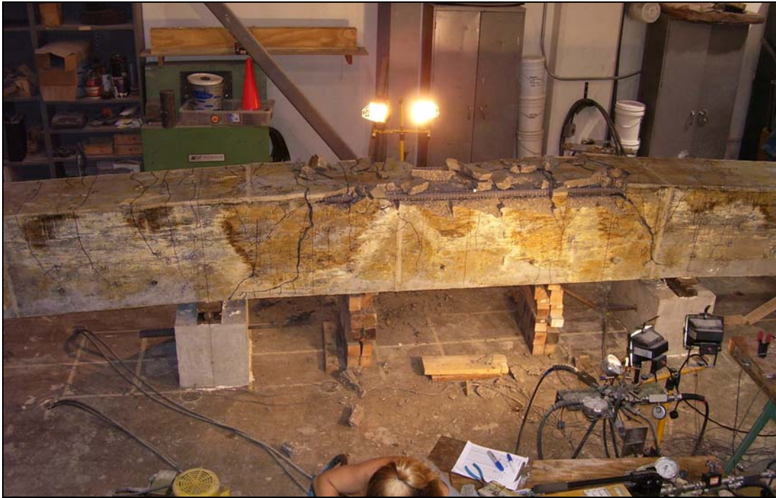
Figure B.35 – Specimen 11-8-XC0-2 at the conclusion of the test
