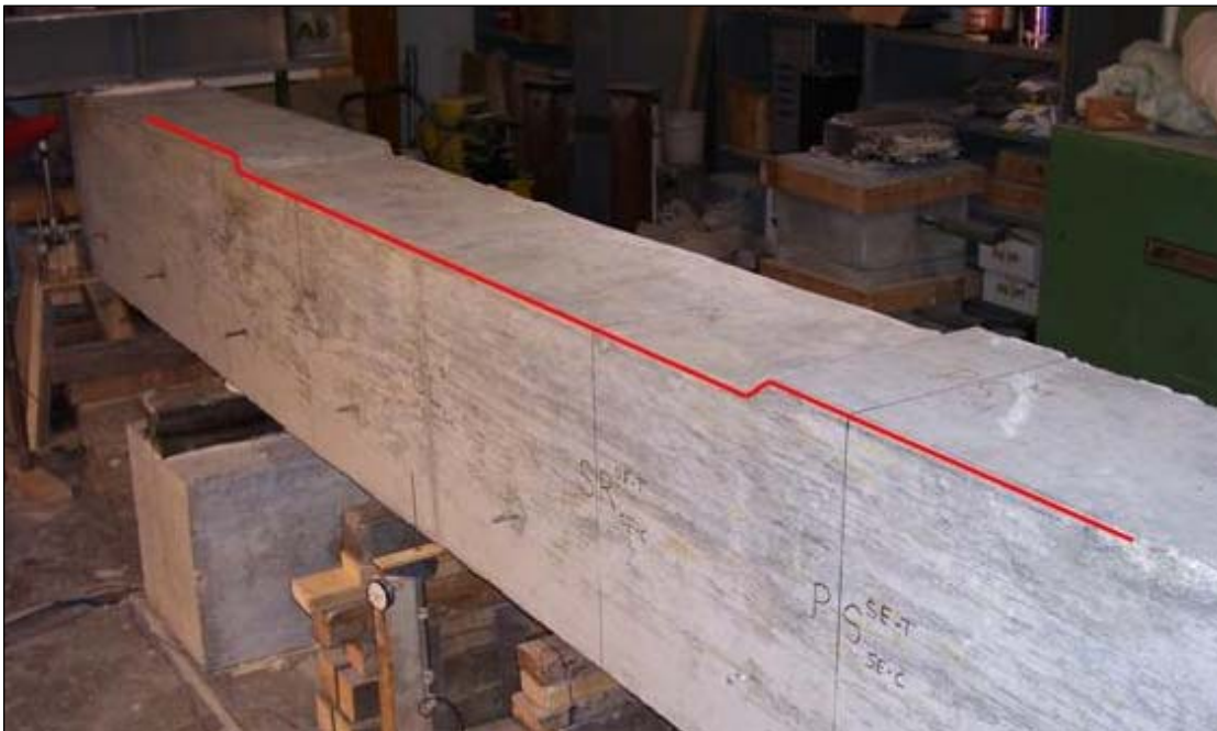
Figure B.1 – Specimen 5-5-XC0-3/4 showing the “dog-bone” reduced section
