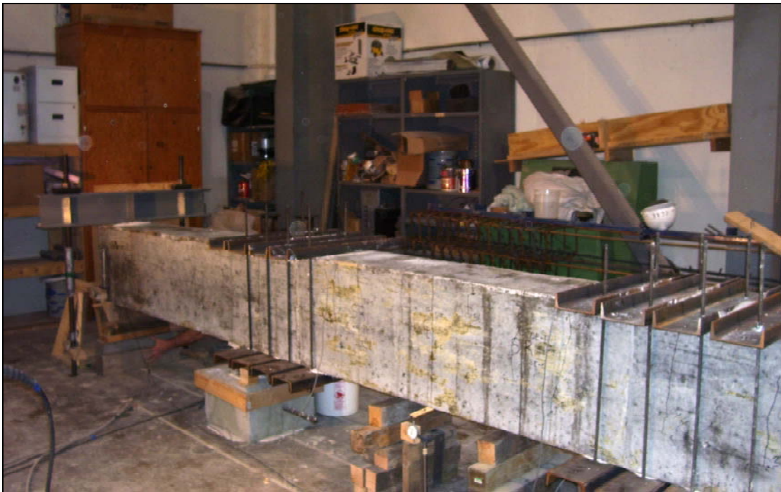
Figure B.26 – External stirrups used to confine specimen 8-8-XC2-2.5
