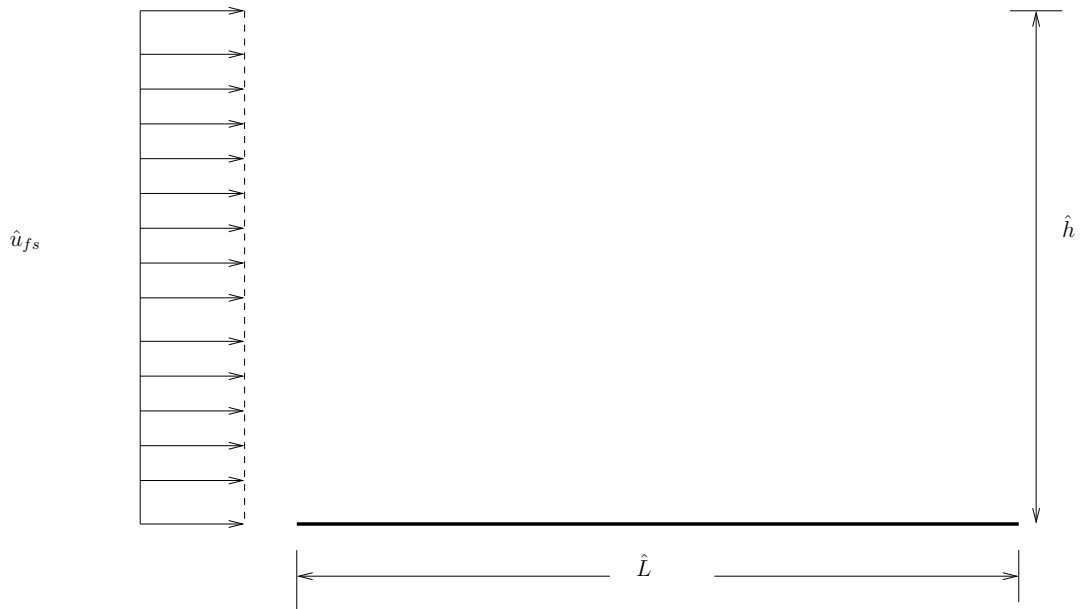
Figure 6.1: Schematic of Carter's plate
