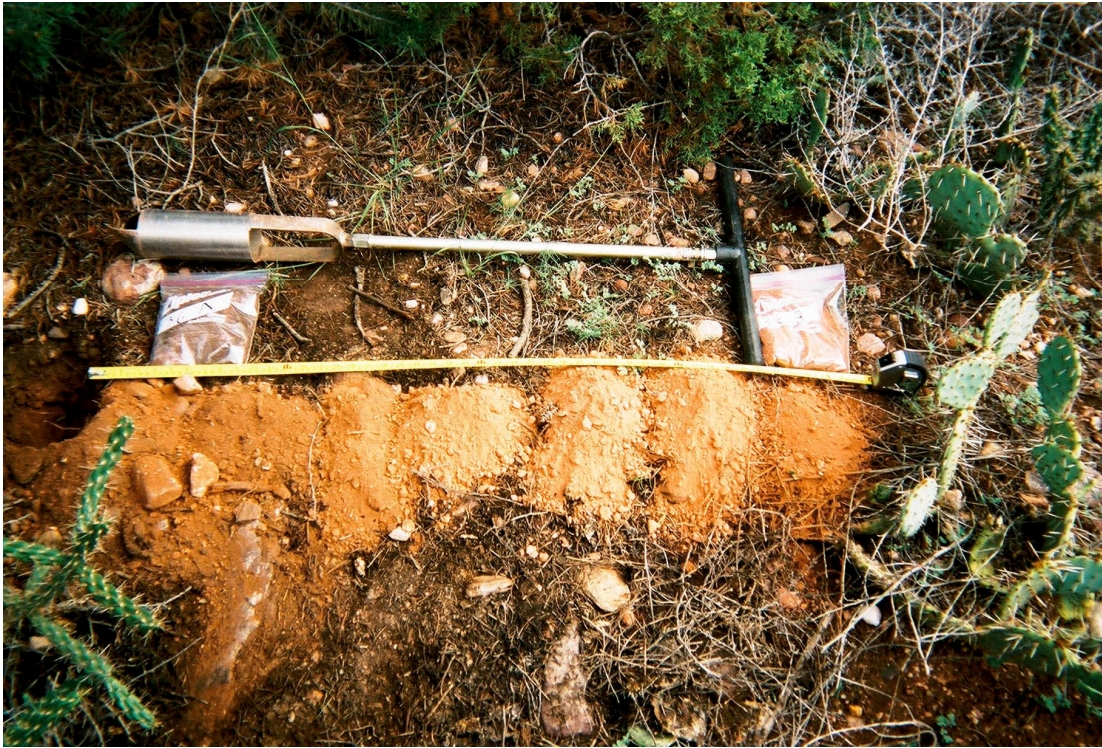
Figure 12. Soil sampling method and materials. Photo by Jeff Krecic.
