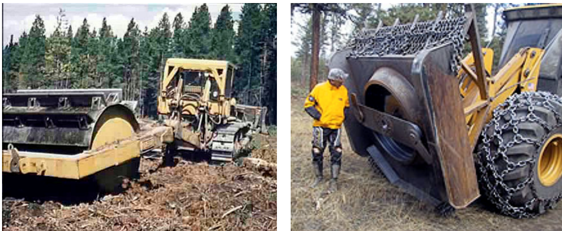
Figure 3. A roller chopper (left) and a hydro-axe (right). Photos courtesy of the Colorado State Forest Service and Cory Cobertt.
