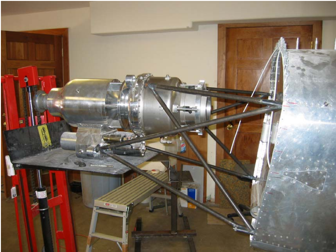
Figure 7.32: Typical Engine Mount for the Innodyn 165TE (Picture courtesy Innodyn, LLC)
