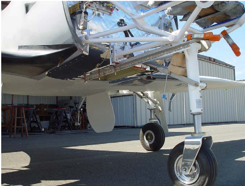
Figure 7.26: Lancair Legacy Landing Gear Installation [50]
