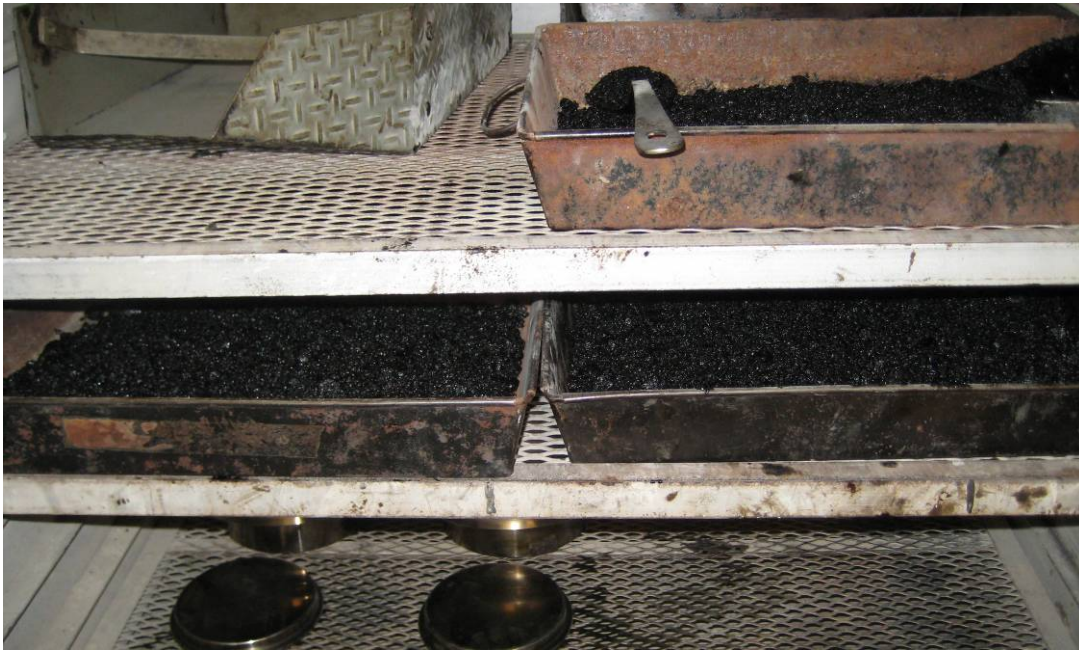
Figure 3-10 Short term aging of Superpave mix
