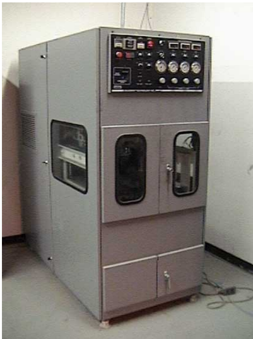
Figure 2-3 Asphalt Pavement Analyzer machine
