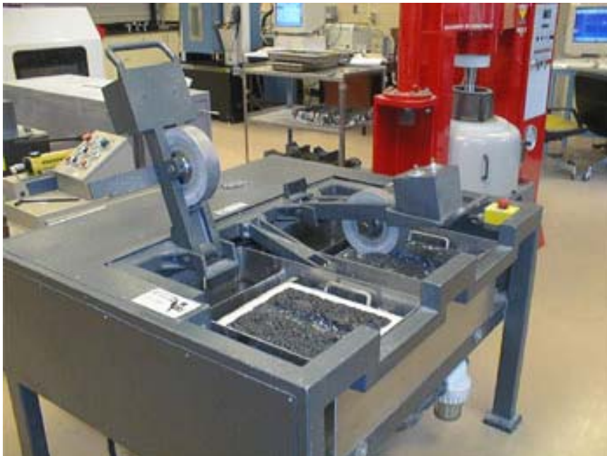
Figure 2-5 Hamburg Wheel Tracking Device
