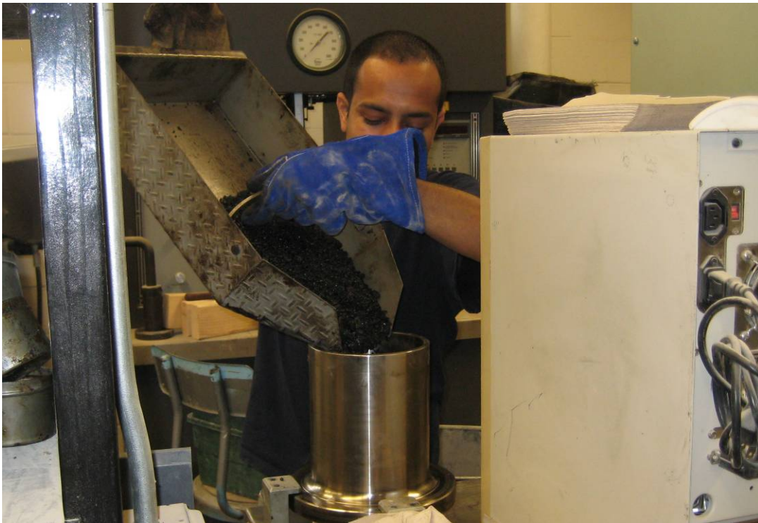
Figure 3-11 Pouring of hot mix in the Gyratory mold.
