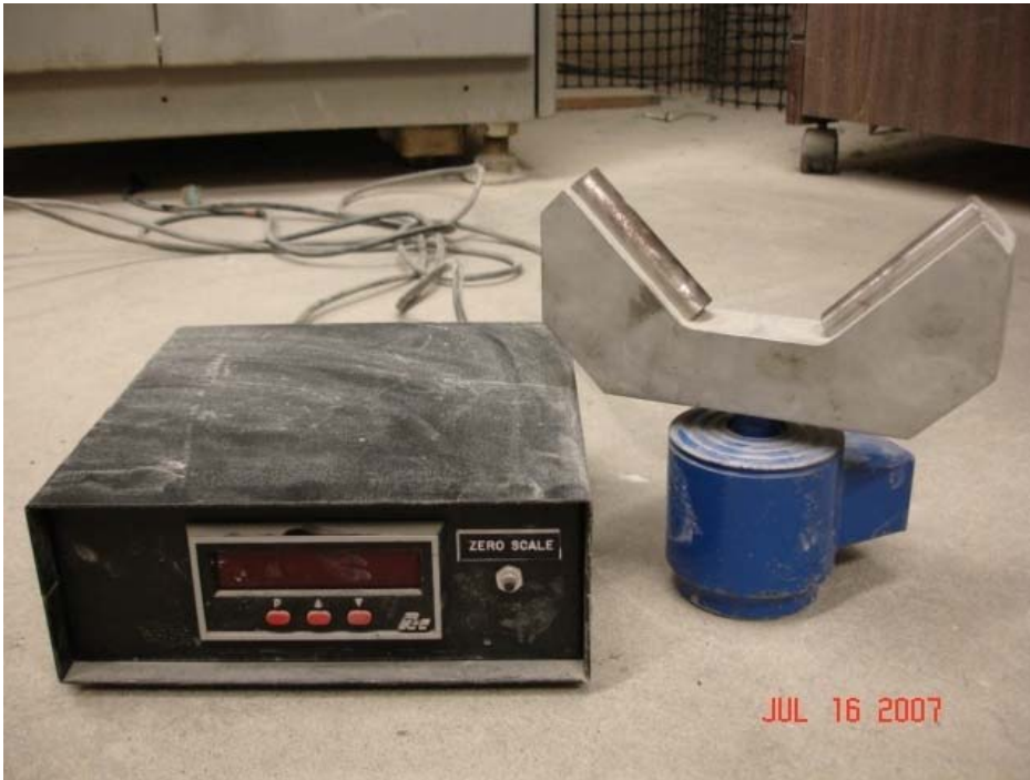
Figure 3-6 Load cell for calibration
