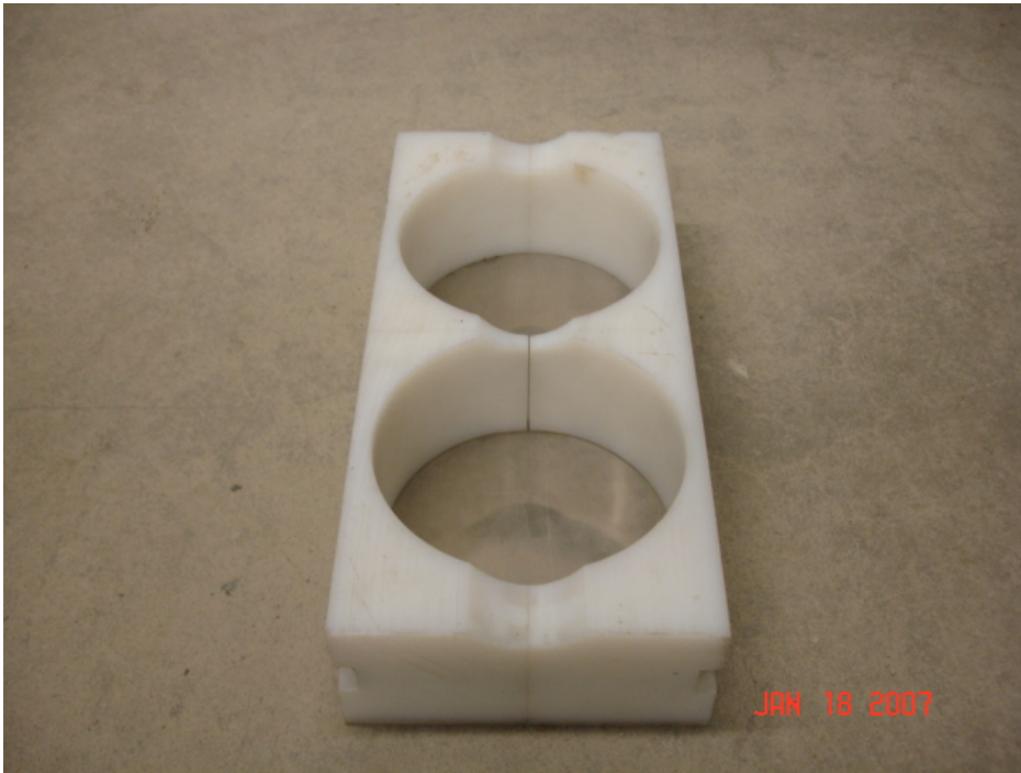
Figure 3-4 Cylindrical mold for rutting tests
