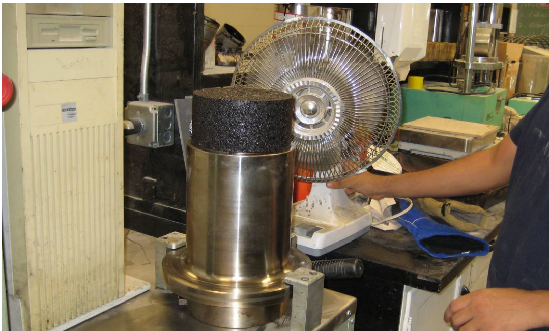
Figure 3-13 Extrusion of the compacted sample from the Gyratory mold
