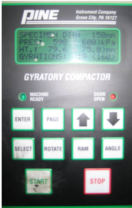
Figure 3-1 Pine Superpave Gyratory Compactor Control Panel
