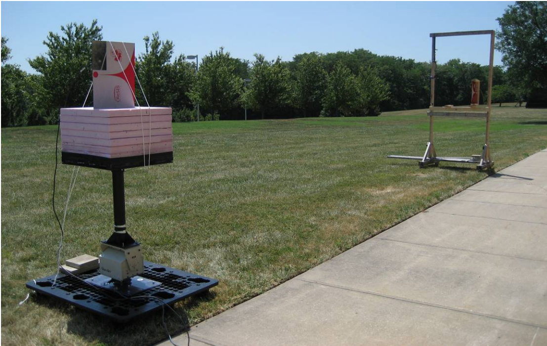
Figure B.5 – H-plane measurement setup
