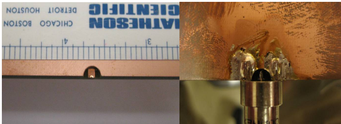
Figure E.2 – Blind via before (left) and after (right) soldering BNC connector
