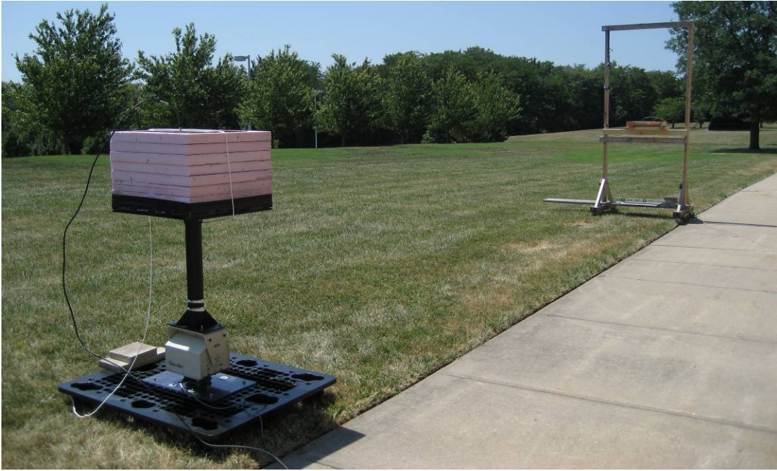
Figure B.4 – E-plane measurement setup
