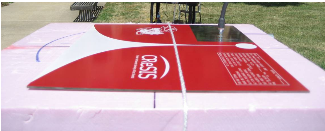
Figure B.2 – Vivaldi under test, E-plane measurement
