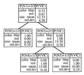
Fig. 3. Concept hierarchy generated by COBWEB/3. The attribute *color* is nominal, and the attribute *size* is assumed to be normal.  $N_1$  is the root node.  $N_2$ ,  $N_4$ , and  $N_5$  are terminal nodes or instances.
