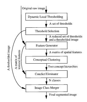
Fig. 1. Block diagram of our segmentation technique.
