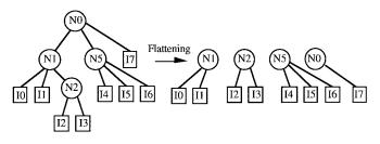
Fig. 6. Process of flattening a hierarchy tree: circles are cluster nodes; boxes are instances.
