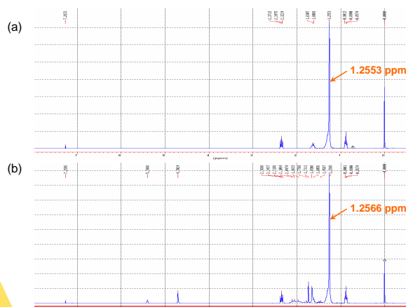
Fig 2. NMR spectra of (a) palmitic acid and (b) equimolar mixture of palmitic acid and limonene in CDCl 3 with TMS.
