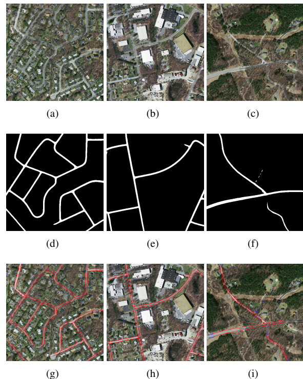
Fig. 1: Upper row: original satellite images; middle row: segmentation results from D-LinkNet34; bottom row: the results of road network extraction by the tube-MPP model.
