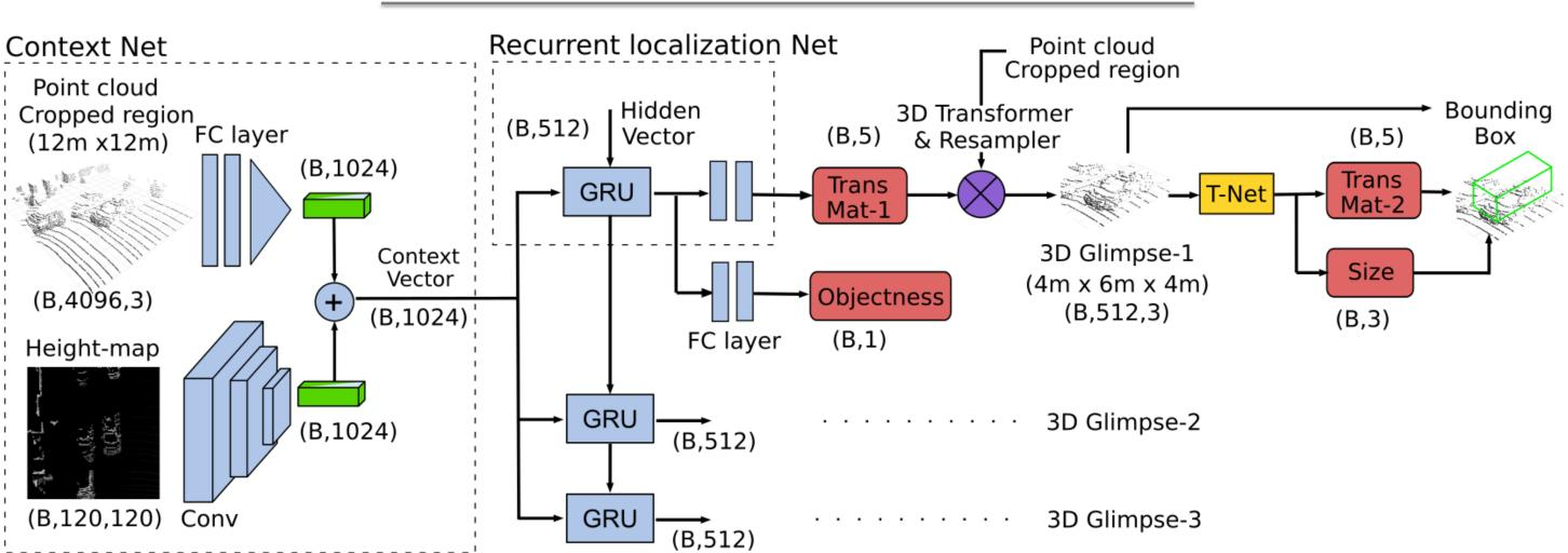
Given the point cloud and the corresponding height map, network sequentially regress parameters of a 3D Transformation matrix representing pose of a fixed size 3D glimpse.
