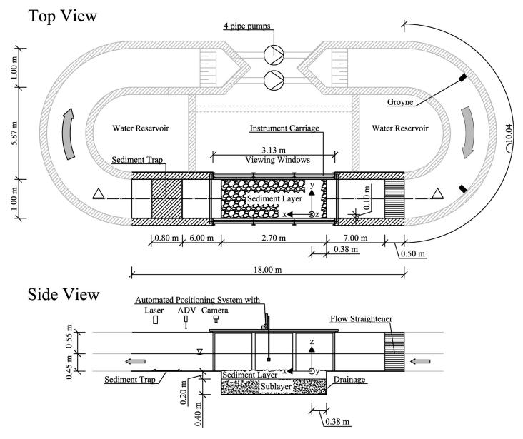
Fig. 1. Schematics of experimental setup in top and side views (not to scale)
