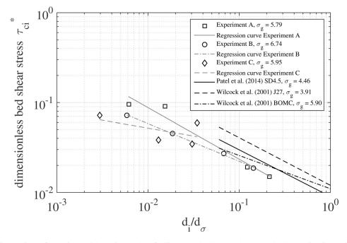
**Fig. 15.** Comparison of experimental data with results of Wilcock et al. (2001) and Patel et al. (2014) with  $d_{\sigma}$  as reference size
