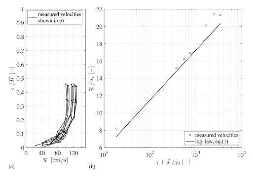
**Fig. 6.** (a) Distribution of time averaged horizontal velocities for Experiment B in the end of Load Case 7, measurement positions are shown in Fig. 4; (b) comparison of measured velocities [gray profile in (a)] and log law;  $u_*$  and  $z_0$  are calculated by applying a logarithmic fit to the measured velocity profiles, the vertical displacement is  $d = 0.25(k_S/3)$  with  $k_S = 30z_0$
