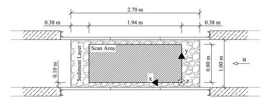
Fig. 5. Bed surface area covered by the laser scanner (1.55 m<sup>2</sup>) in relation to the total dimensions of the material bed (2.70 m<sup>2</sup>)
