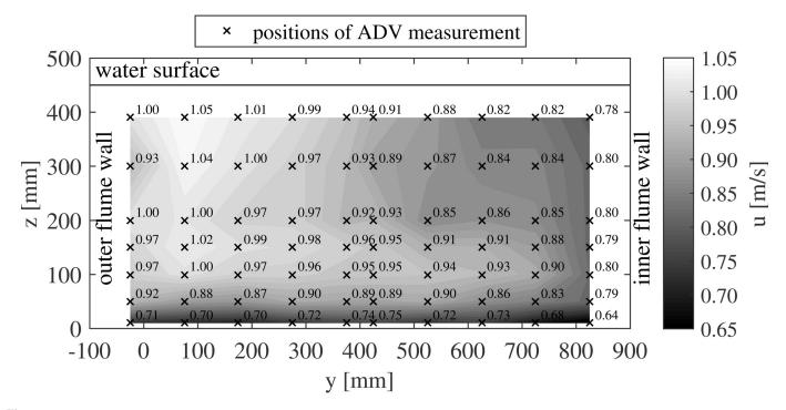
**Fig 3.** Distribution of time-averaged flow velocities in meters per second over the flume width y during preliminary testing for the highest load case (mean  $\bar{u} = 0.9 \text{ m/s}$ ); the velocities were measured 1 m upstream of the sediment bed
