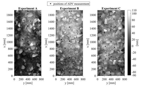
Fig. 4. Digital elevation models of initial bed surface for the three experiments; flow direction is from the bottom to the top
