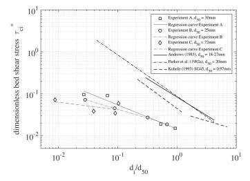
**Fig. 14.** Comparison of experimental data with results of Andrews (1983), Parker et al. (1982b), and Kuhnle (1993) with  $d_{50}$  as reference size
