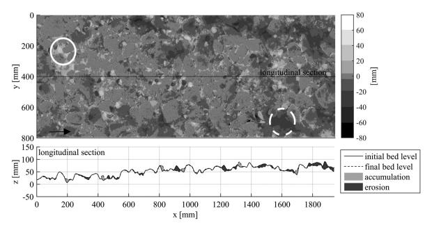
**Fig. 10.** Erosion (dark gray) and accumulation (light gray) areas at the end of Experiment B; full-lined circle indicates typical accumulation of finer fractions behind larger stones, and dash-lined circle indicates extensive erosion of finer fractions in unprotected areas
