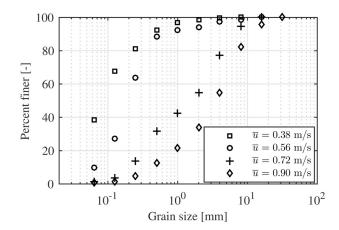
**Fig. 8.** Grain size distributions of eroded bed load collected by the sediment trap for the last four load cases in Experiment B
