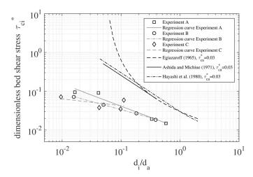
**Fig. 13.** Comparison of measured dimensionless critical shear stresses  $\tau_{c,i}^*$  with approaches of Egiazaroff (1965), Ashida and Michiue (1971), and Hayashi et al. (1980) with  $d_a$  as reference size
