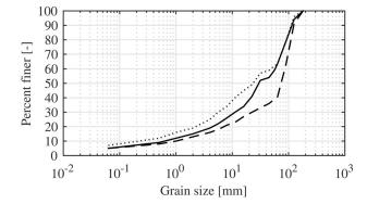
**Fig. 2.** Grain size distributions of investigated wide-graded material samples
