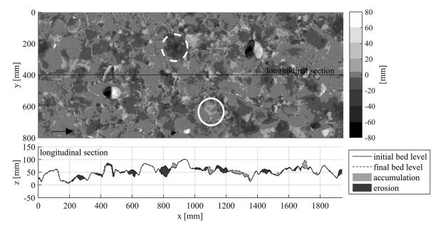
**Fig. 11.** Erosion (dark gray) and accumulation (light gray) areas at the end of Experiment C; full-lined circle indicates typical accumulation of finer fractions behind larger stones, and dash-lined circle indicates extensive erosion of finer fractions in unprotected areas
