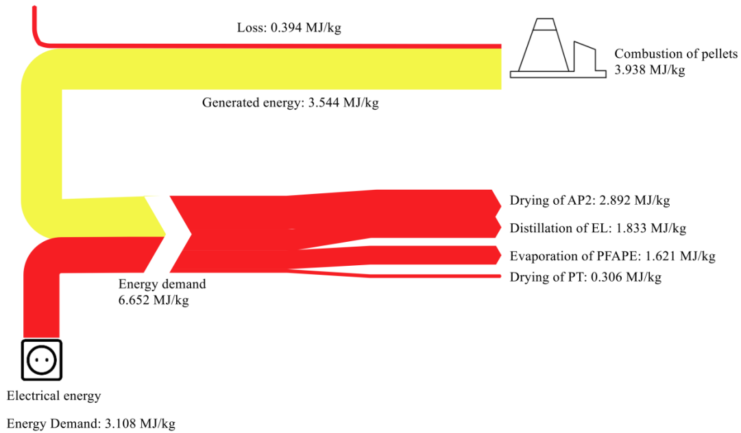
Figure 6.5 Heat balance in the production of pectin, pellets and pectin free apple pomace extract in MJ/kg AP1
