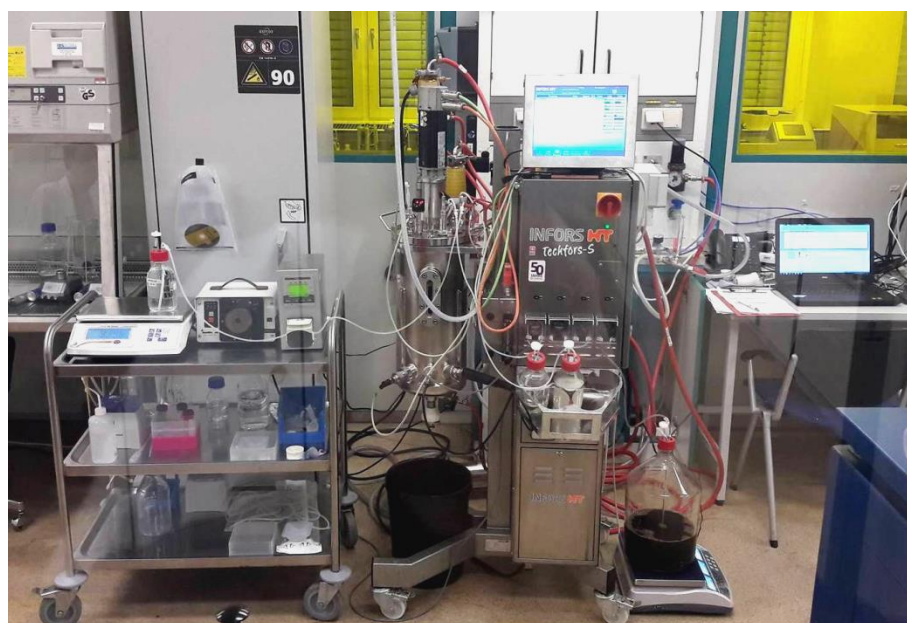
Figure 4.3 Pilot scale set up for conducting fed-batch fermentations
