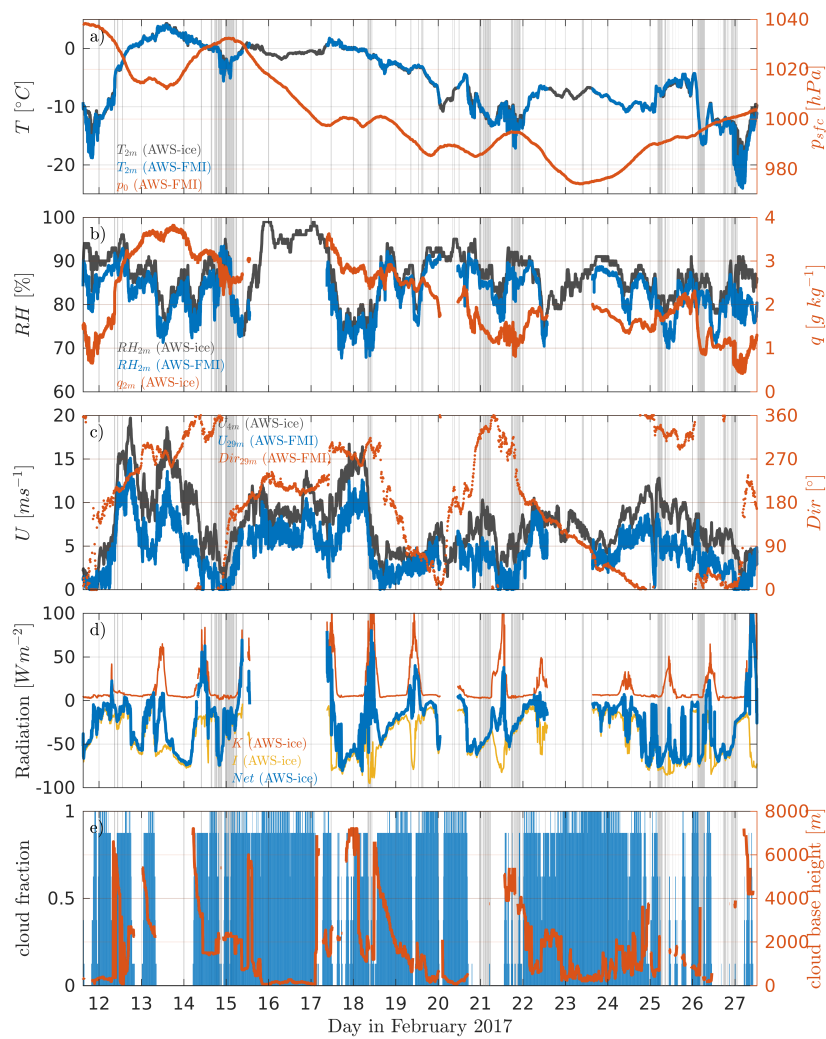
Figure 6. Overview of the meteorological conditions: (a) temperature, T , and surface pressure, p ; (b) relative, RH , and specific humidity, q ; (c) wind speed, U ; and direction, Dir ; (d) short-wave, K , long-wave, I , and net radiation balance, Net ; (e) total cloud fraction and cloud base height. Gray shading indicates times of UAV operation. Note that the wind measurements over land were performed at 29 m above ground.
