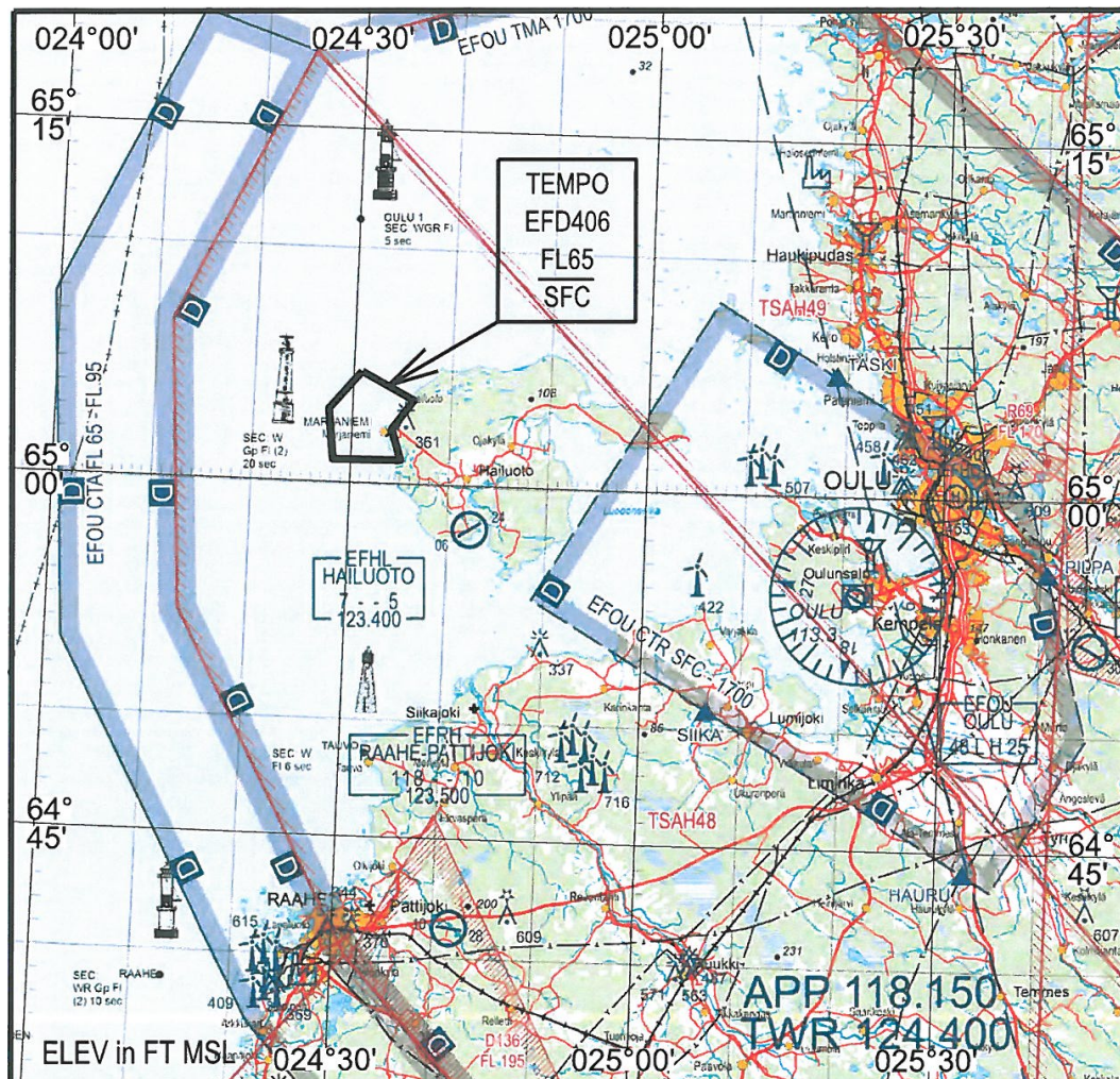
Figure 3. Aviation map of the area around Oulu airport. The danger area reserved for our UAV operations is outlined in bold and labeled as TEMPO EFD406 (Source: ANS Finland Aeronautical Information Services AIP Supplement Map).
