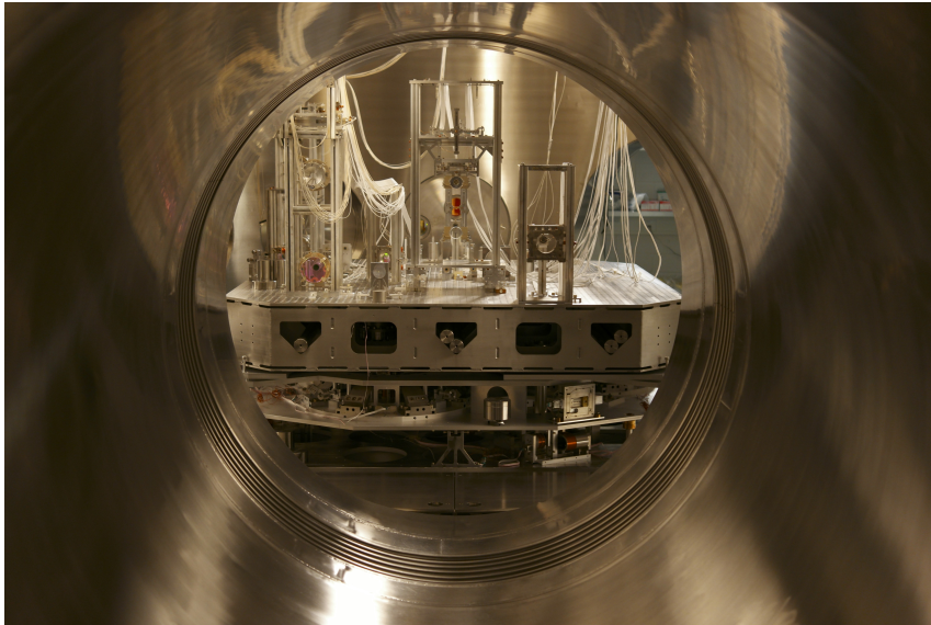
(a) View from the center of the south tube onto the south optical bench. On the right the 3" collimating mirror and in the center the end mirror of the Single Arm Test are installed.
