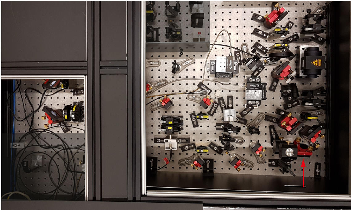
Figure 2.4: Picture of the newly setup laser preparation. The setup was compacted to allow space for other experiments, such as the optical lever. The consumed laser power was reduced from 500 mW to 200 mW. The laser itself is located in the bottom of the picture. A simplified sketch of the laser preparation can be found in figure 2.1.
