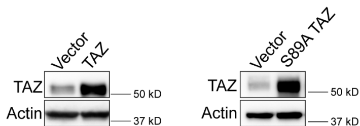
Figure 2.12. Expression of Wild-Type and S89A TAZ Constructs. MDA-MB-231 cells were transfected with empty vector, wild-type TAZ or S89A TAZ and processed for immunoblotting.
