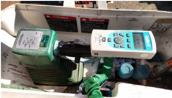
Figure 3. Chatillon™ force gage attached to the pistol grip control to measure forward/rearward force. A 3D printed clamshell (black) was secured to the pistol grip to provide a secure mount for the Chatillon™ gage.
