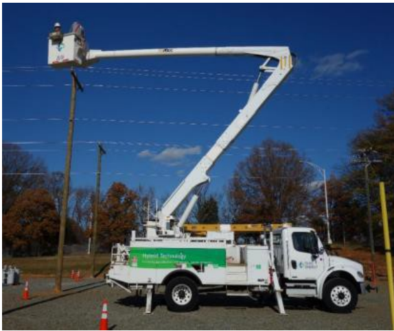
Figure 1. Typical electric utility aerial bucket truck with a 2-segmented boom.
