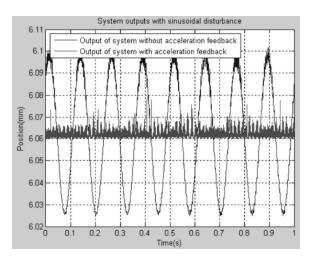
Fig. 12. System outputs of a maglev system subject to a sine disturbance
