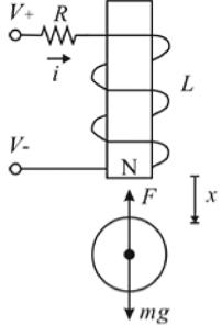
Fig. 2. Free body diagram of the maglev system
