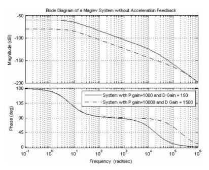
Fig. 6. Bode diagram of a maglev system with different controller gains
