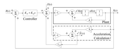
Fig. 10. Block diagram of a maglev system with acceleration feedback
