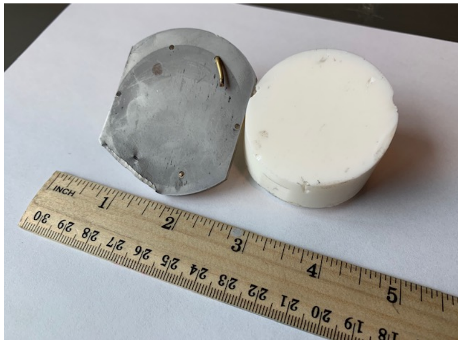
Fig. 6-4. Recovery impactor and target anvil from a polyurethane dynamic friction oblique impact experiment. Edge damage is mostly likely from secondary impacts/interactions inside the catch tank experiment duration. The impact site is observable and evidence of smearing suggests slip did occur.
