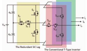
Fig. 2 The proposed fault-fault three-level T-type inverter topology.
