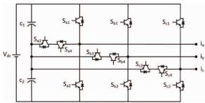
Fig. 1 Conventional three-phase three-level T-type inverter topology.
