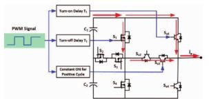
**Fig. 4** Quasi ZVS and ZCS switching strategy during positive output voltage of the phase-A leg of the T-type inverter at positive output current condition.
