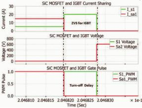
**Fig. 7** Current sharing and ZVS switching between SiC MOSFET ( $S_1$ ) and IGBT ( $S_{a2}$ ) under positive output voltage and positive output current condition of the T-type inverter.
