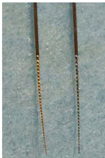
Figure 2. Titanium nitride coated (gold color; left) and uncoated endodontic files.
