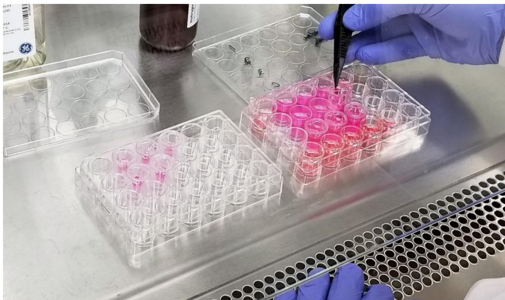
Figure 8: The transfer of inserts and media to new wells as part of the cell proliferation test protocol
