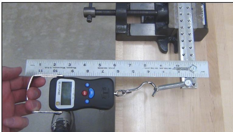
Figure 6. Spring rate measurement setup.
