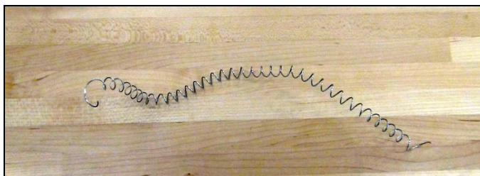
Figure 7. An overextended spring.
