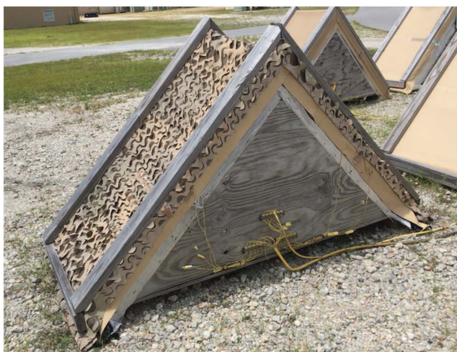
Fig. 5. Test jig configured with all three layers spaced 1.5 inches apart.
