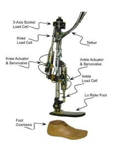
Figure 2.12: Knee and Ankle Prosthesis with Major Components [41]
