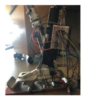
Figure 6.2: Side View of Marquette Prosthesis II with Hardware Attached
