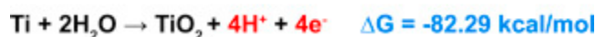
Fig. 3. Oxide layer formation. Ti spontaneously reacts with air and water to form a thin layer of oxide ( \text{TiO}_2 ) at the surface
