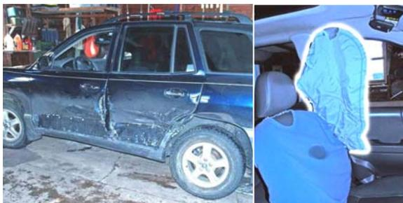
Figure 6. Case 3 vehicle damage and SAB.
