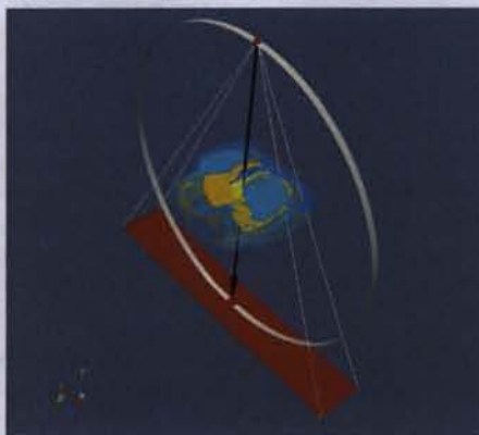
Figure 1: Scan geometry. The thorax was cropped to 31 cm by 22 cm in the lateral and anteroposterior directions, respectively, and 30 cm in the axial direction. The first view angle of the scan is AP (arrow). The detector measures 100 cm laterally 16 cm axially (rectangle).
