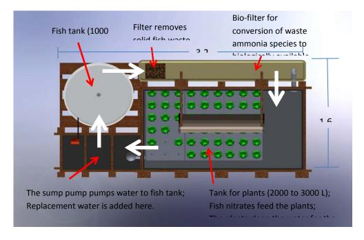
Figure 2. Top view of a small aquaponics system with descriptions of components. The white arrows represent the flow of water.
