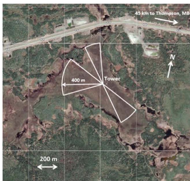
Figure 1. Layout of the BOREAS NSA fen site, after Lafleur et al. [1997]. Sectors identifying acceptable wind directions and approximate source area represented in tower-based flux measurement. Image copyright GeoEye, obtained through Google Earth ( www.google.com ).
