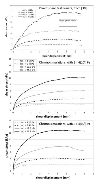
Fig. 3 Direct shear test results for 5000 randomly packed uniform glass beads obtained by experiment [30] (top) and DEM-PM simulations using Chrono (center and bottom), under constant normal stresses of 3.1, 6.4, 12.5, and 24.2 kPa. For the DEM-PM simulations, elastic moduli of  $E = 4(10^6)$  Pa (center) and  $E = 4(10^7)$  Pa (bottom) are used.
