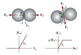
Fig. 1 DEM-PM contact model described in this section, with normal overlap distance  $\delta_n$ , contact-normal unit vector n, and tangential displacement vector  $\mathbf{u}_t$  in the plane of contact (top), and with a Hookean-linear contact force-displacement law with constant Coulomb sliding friction (bottom)
