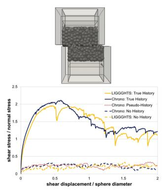
Fig. 2 Direct shear simulation setup (top) and shear versus displacement results (bottom) obtained by Chrono [14] and LIGGGHTS [15] for 1800 randomly packed uniform spheres using the true tangential contact displacement history model of Eq. (4), the pseudohistory model of Eq. (5), and no tangential contact history
