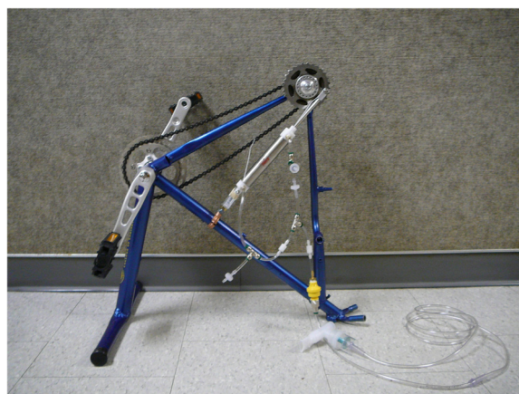
Figure 2 Bicycle compressor. The bicycle design of the HPN is a stationary single bi-directional piston design. This prototype device was constructed from a commercially available bicycle frame. The frame was cut and re-welded to produce the device. The silver cylinder is a bi-directional piston attached to the frame and the gear. The white plastic pieces are the one-way valves configured in the manner indicated in Figure 1, and the yellow plastic piece is the flow regulator. The nebulizer mouthpiece and tubing is connected to the output of the flow regulator. The operator—who is someone other than the patient—sits in a chair and pedals the device by foot. The effort required is roughly equivalent to riding a bicycle at a rate of eight miles per hour.
