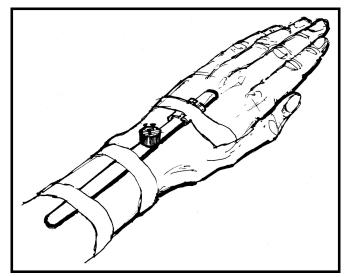
Figure 4. Wrist monitor that measured wrist radial and ulnar deviation.
