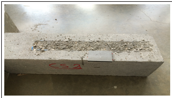
Figure 12. Concrete substrate surface after FRP debonding in shear pull-out test.
