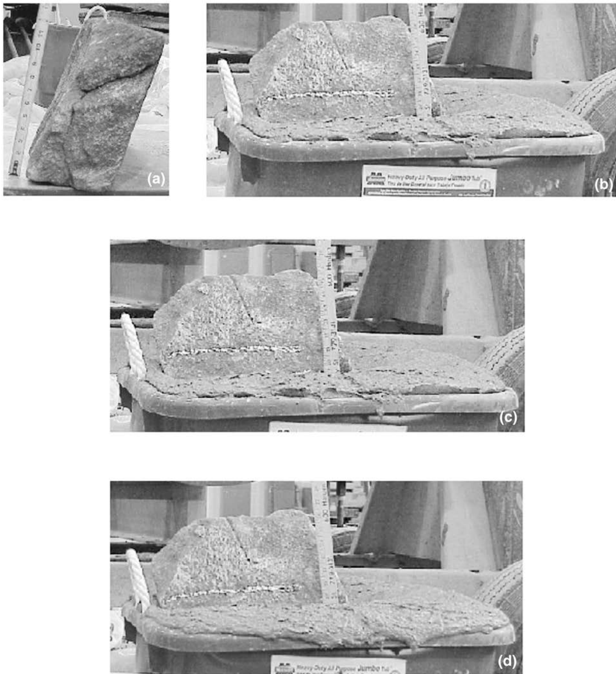
Fig. 4—Experimental setup of large stone placed on fresh mortar.
