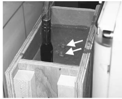
(b) test specimen at initiation of vibration showing metallic spheres at mortar surface (only two spheres can be seen)
