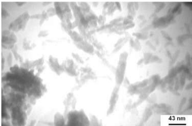
Fig. 1. Transmission electron micrograph of the synthesized nanostrontium hydroxyapatite.
